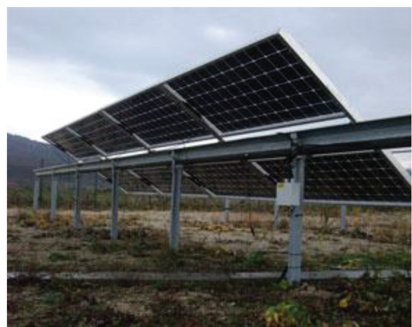
Figure 6. Commercial open-field installation in Saxony, Germany: 8 months with a 20% (0.2) reflectance ground albedo and 12 months with a 50% (0.5) reflectance ground albedo. Results: 17% bifaciality gain over the best module in the field and more than 60% gain in snowy conditions. (The bifacial system kept collecting solar energy through the back side even when the front side was covered with snow, in contrast to all the other systems, which stopped yielding power in these conditions.) The respective cell equivalent efficiency values are 21.7% and 29.6% [13].
