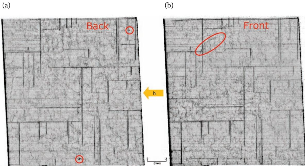
**Figure 12.** Depth-selective images from the QC-TT, generated from the same measurement data set: (a) back of a mono-like Si sample; (b) front of the sample. The red ellipses indicate some features which are not common to the two images and therefore arise from defects located at or near the respective surfaces.
