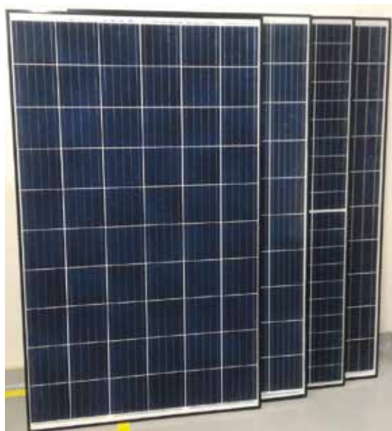
Figure 7. Photographs of fabricated sample PV modules (5-BB LTR, 6-BB, 5-BB halved-cell, 3-BB).
