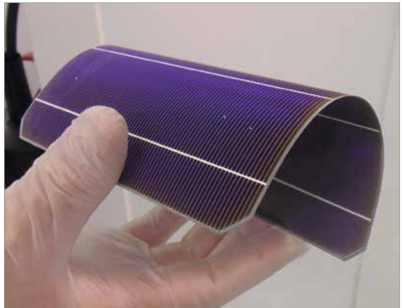
Figure 6. Flexibility of a 60µm SHJ bifacial cell (156mm × 156mm).
