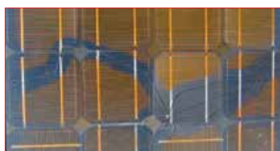
Figure 9. Photograph of a module after extended outdoor exposure at JRC (Italy) showing strong browning caused by photo degradation of the EVA and bleaching effects around the cracks in the cover glass. (This module is unrelated to other modules investigated in this project.)
