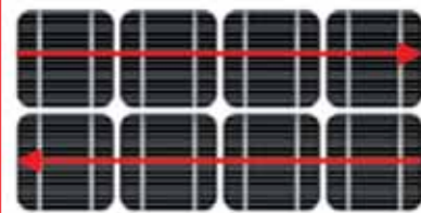
Figure 3. Illustration of the scan path across the PV modules.
