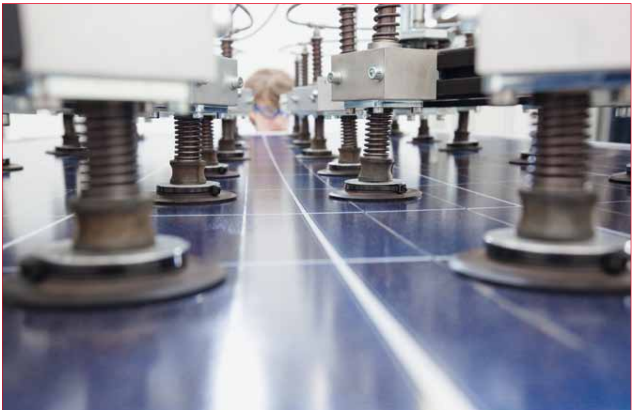
Figure 2. Load testing at the Hanwha Q CELLS test centre.
