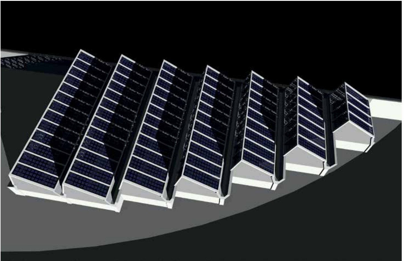
Figure 2. A rendered image of the BIPV system shown in Fig. 1 based on a RADIANCE model. Partial shading of the system at this specific time step is clearly visible [3]
