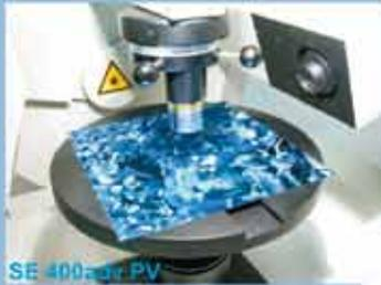
Laser ellipsometer and spectroscopic ellipsometer for measurement of thickness and refractive index of AR coatings on textured multi-crystalline and mono-crystalline silicon wafers.
