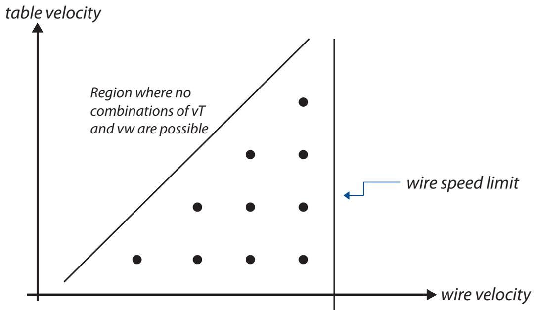
Figure 3. Free abrasive slurries are restricted by limits of rates at which the wire can deliver work energy to the slot. As silicon load and system power increases, table speeds must be lowered due to rising entropic losses which further reduces the work energy delivery rate.
