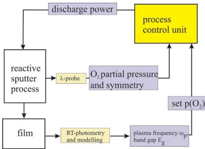
Figure 6. Schematic of the closed loop of the online control. The first cycle (top loop) controls oxygen partial pressure during deposition by adjusting power, and the symmetry by adjusting the flow. The second cycle (bottom loop) controls the deposited film properties by adjusting the set point for  $p(\text{O}_2)$  via taking optical measurements and curve fitting.
