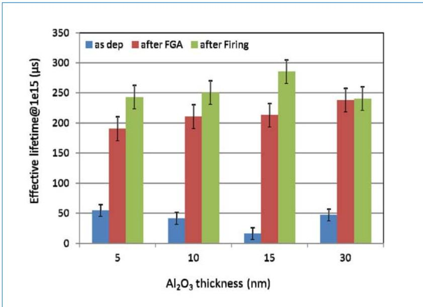
Figure 4. Thermal stability of different Al<sub>2</sub>O<sub>3</sub> thicknesses on *p*-type CZ (2Ωcm), with SDR and polishing prior to passivation.
