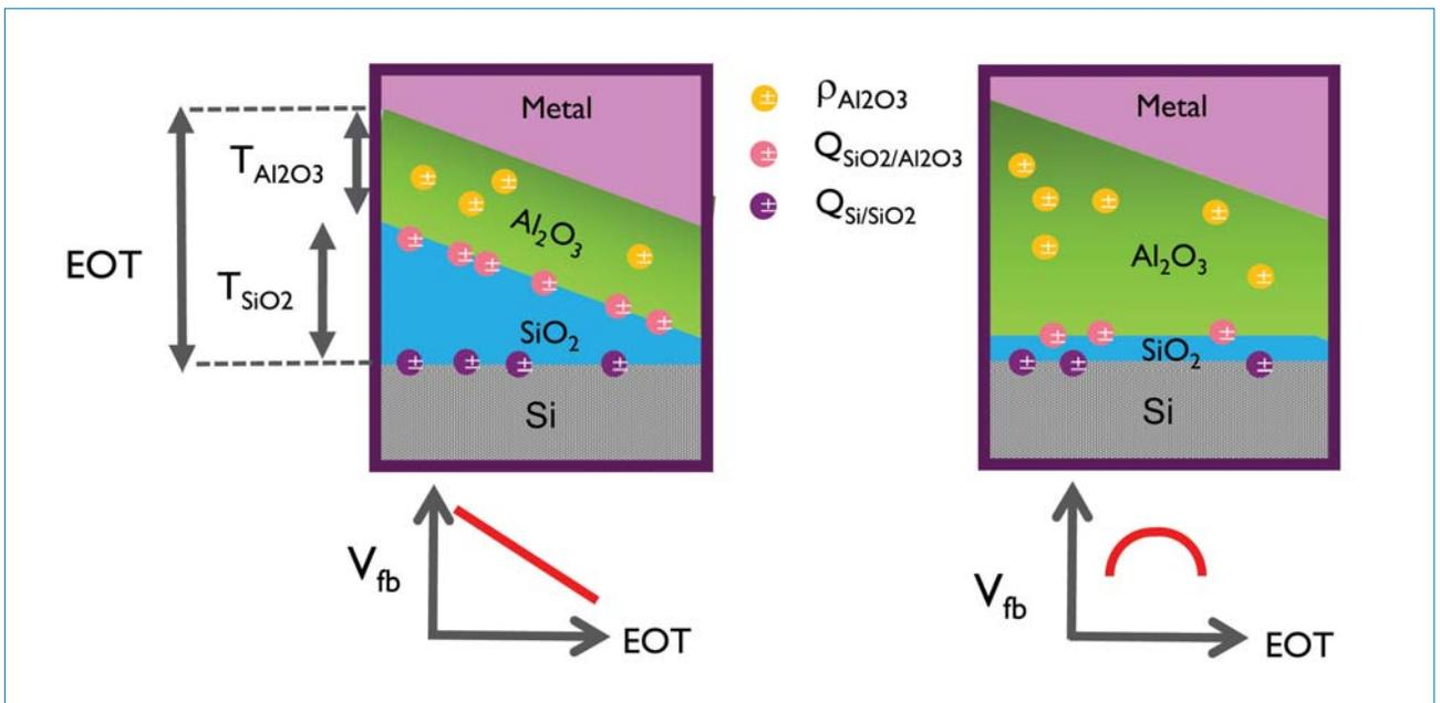
Figure 5. Charge extraction model – double-thickness series approach for determination of fixed charge within the passivation stack (Si/SiO<sub>2</sub>/Al<sub>2</sub>O<sub>3</sub>): (a) varying only SiO<sub>2</sub> thickness enables Q<sub>Si/SiO<sub>2</sub></sub> extraction; (b) varying only high-k thickness enables Q<sub>SiO<sub>2</sub>/Al<sub>2</sub>O<sub>3</sub></sub> and ρ<sub>Al<sub>2</sub>O<sub>3</sub></sub> extraction.
