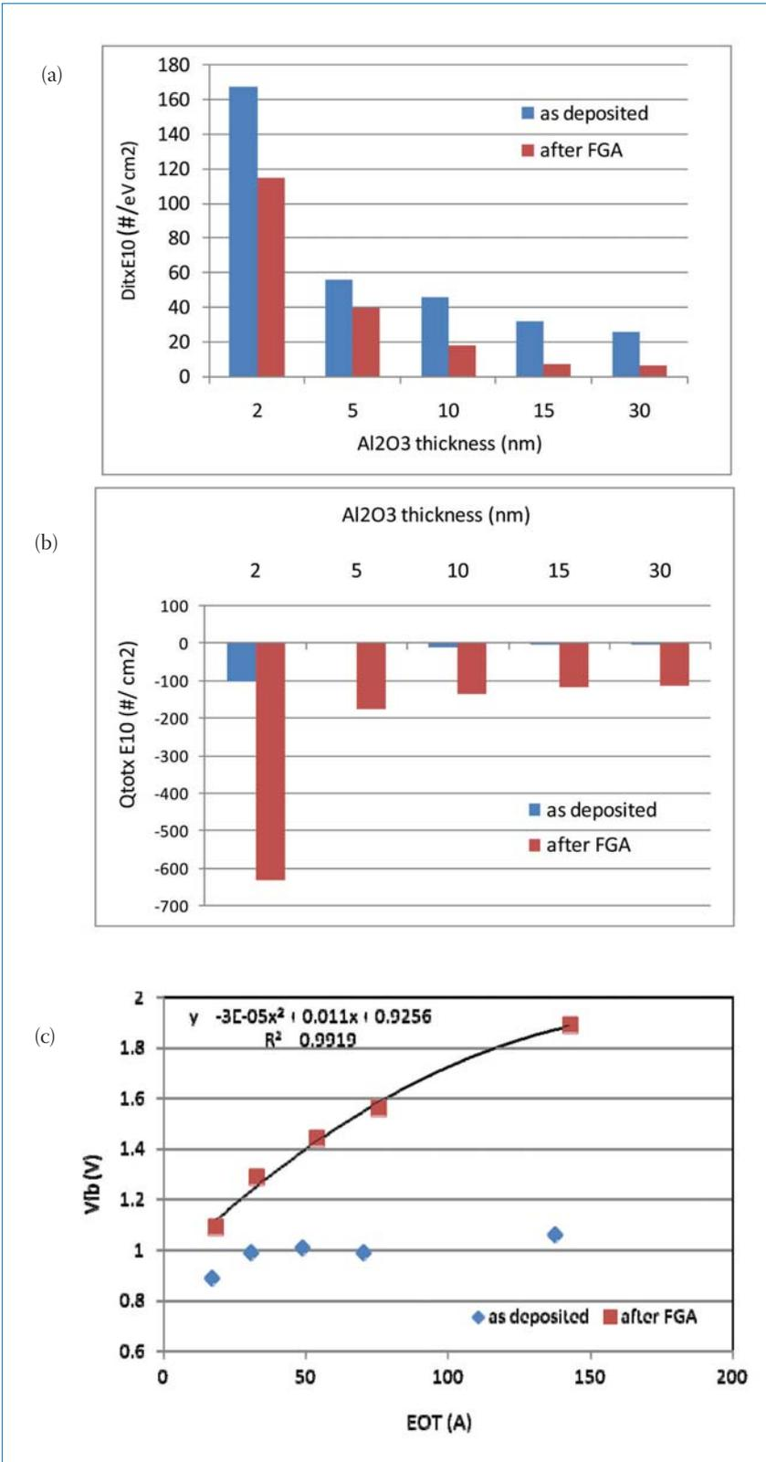
Figure 6. (a) Interfacial trap density  $D_{it}$  and (b) total amount of charge  $Q_{tot}$  extracted from  $V-Q$  measurements for Al<sub>2</sub>O<sub>3</sub> as deposited and after FGA@350°C; (c) flat-band voltage versus equivalent oxide thickness EOT for Al<sub>2</sub>O<sub>3</sub> as deposited and after FGA@350°C. The annealed samples exhibit a positive slope, indicating the presence of a global negative charge build-up within the c-Si/SiO<sub>2</sub>/Al<sub>2</sub>O<sub>3</sub> stack.
