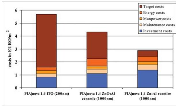
Figure 8. Comparison of typical cost-of-ownership calculations for ITO, ZnO:Al (ceramic process), and ZnO:Al (reactive process)[21].
