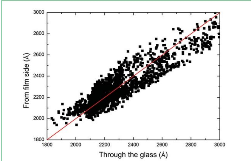
**Figure 15.** Correlation between the CdS thickness determined in a film-side measurement and the corresponding results obtained at the same position but through the glass. The scatter plot is obtained from individual measurements over the  $40 \times 80\text{cm}^2$  region of the CdS-coated TEC-15 glass plate of Figs. 12–14.
