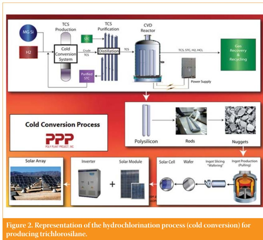
Figure 2. Representation of the hydrochlorination process (cold conversion) for producing trichlorosilane.
