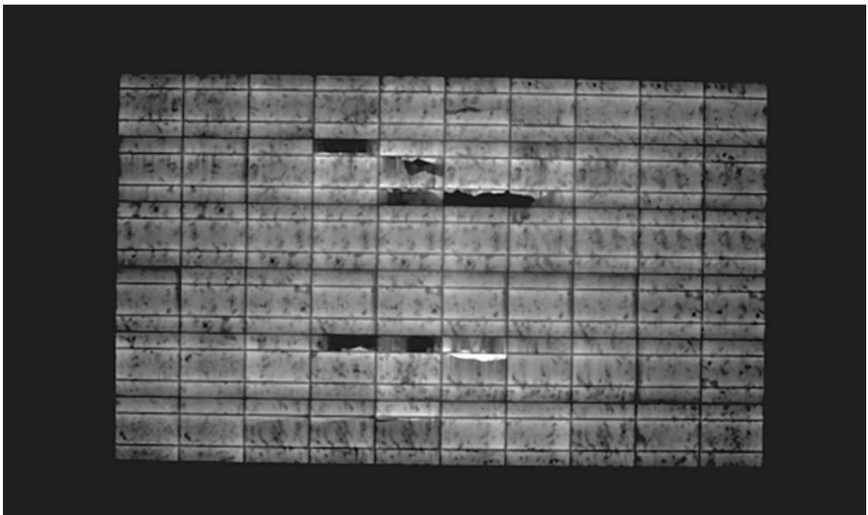
Figure 4. Electroluminescent imaging of a multicrystalline module.
