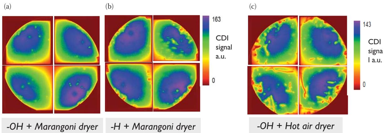
Figure 1. Comparison of passivation levels reached after annealing for different surface preparations before ALD- $\text{Al}_2\text{O}_3$  deposition: a) -OH terminated + Marangoni; b) -H terminated + Marangoni; c) -OH terminated + hot air dryer. Lifetime measurements were performed by carrier density imaging (CDI).
