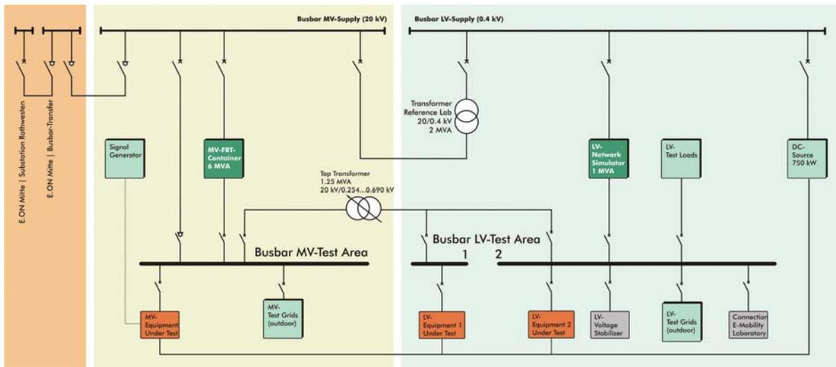
Figure 3. Schematic of the new reference laboratory of Fraunhofer IWES at IWES-SysTec for testing DER units in the higher power range.
