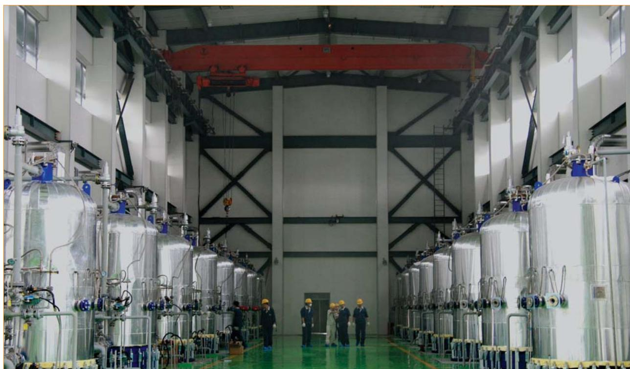
Figure 3. CVD reactors in the polysilicon plant deposition building.
