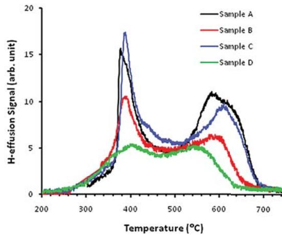
Figure 6. Hydrogen-effusion time profiles for four different nc-Si:H solar cells. Samples A and C have low crystalline volume fraction, while B and D are highly crystalline.
