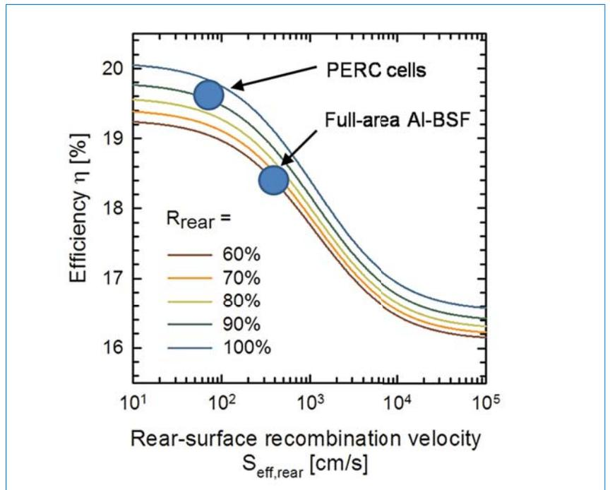
Figure 4. PC1D simulation of the conversion efficiency η vs. the rear-surface recombination velocity S<sub>eff,rear</sub> for different internal rear reflectance values R<sub>rear</sub>. Whereas the full-area Al-BSF of typical industrial-type silicon solar cells with S<sub>eff,rear</sub> = 400cm/s and R<sub>rear</sub> = 65% limits the conversion efficiency to ~18.5%, screen-printed PERC cells with dielectric rear passivation have the potential to achieve 20% conversion efficiency.
