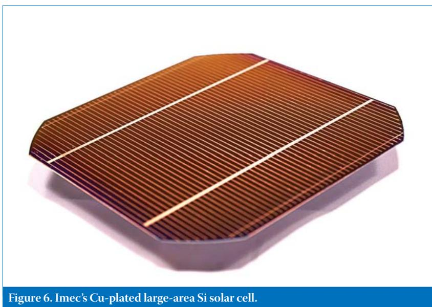
Figure 6. Imec’s Cu-plated large-area Si solar cell.
