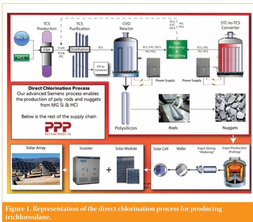
Figure 1. Representation of the direct chlorination process for producing trichlorosilane.
