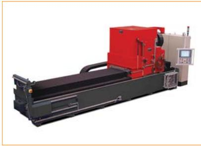
**Arnold's squaring saw uses two diamond cutting discs for monocrystalline brick production**
