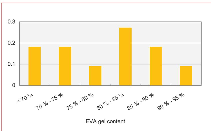
Figure 7. Frequency distribution of EVA gel content of analyzed solar modules from manufacturer A.
