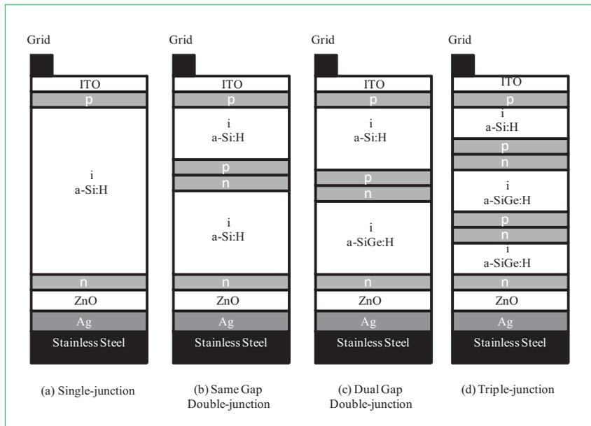
Figure 2. Schematic of different cell structures.
