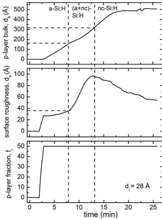
**Figure 9.** Evolution of bulk layer thickness (top), surface roughness layer thickness (centre) and interface filling fraction (bottom) during roll-to-roll PECVD of a thin-film Si:H *p*-layer at  $v = 0.015\text{cm/s}$  web speed on an underlying a-Si:H *i*-layer. In the bottom panel, a transition from *i*-layer surface roughness to *i/p* interface roughness occurs when the *p*-layer filling fraction reaches 50 vol%.
