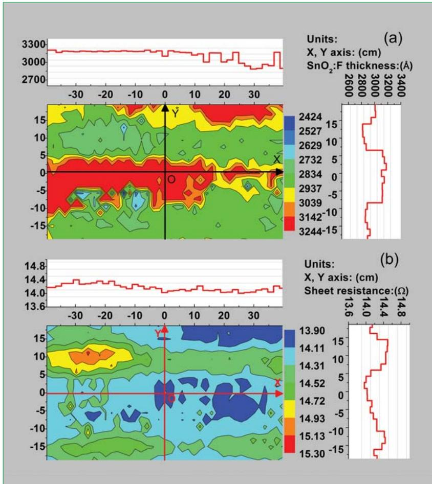
Figure 14. Maps of (a)  $\text{SnO}_2\text{:F}$  bulk layer thickness on the TEC-15 glass panel and (b) optical sheet resistance of the  $\text{SnO}_2\text{:F}$  layer. The plate in this case is the same as the one in Figs. 12 and 13; thus the  $\text{SnO}_2\text{:F}$  layer lies beneath the CdS layer. The plots in (a) and (b) (above and to the right of the maps) show the variations in the deduced parameters along the X and Y axes.
