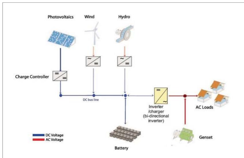
Figure 2. Examples of mixed-source rural electrification solutions.
