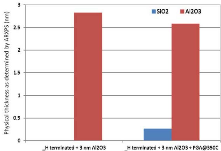
Figure 2. Interfacial  $\text{SiO}_2$  regrowth is observed on a hydrophobic surface after annealing c-Si/3nm  $\text{Al}_2\text{O}_3$  by FGA@350°C.
