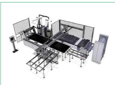
**Gerold's HMA-system offers automatic hot melt edge-sealing of thin-film modules**
