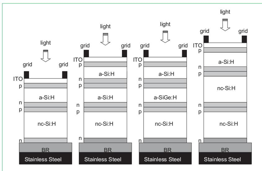
Figure 4. Different cell structures incorporating nanocrystalline silicon.
