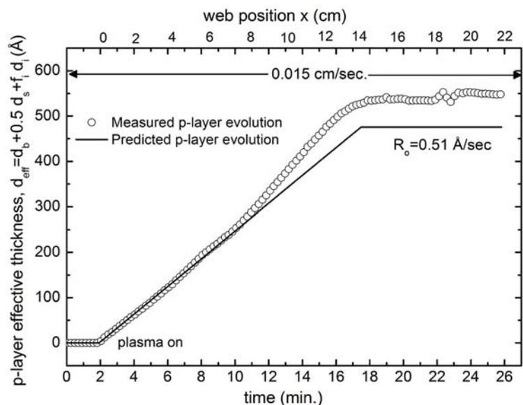
Figure 8. Evolution of the effective thickness as measured by SE during roll-to-roll deposition of a thin hydrogenated silicon (Si:H) *p*-layer at a web speed of  $v = 0.015\text{cm/s}$  on an underlying a-Si:H *i*-layer; also shown is a prediction (solid line) assuming a time- and position-independent deposition rate  $R_0$  within the plasma zone. The assumed rate of  $R_0 = 0.51\text{\AA/s}$  is that associated with an amorphous phase as measured in the early stages of growth.
