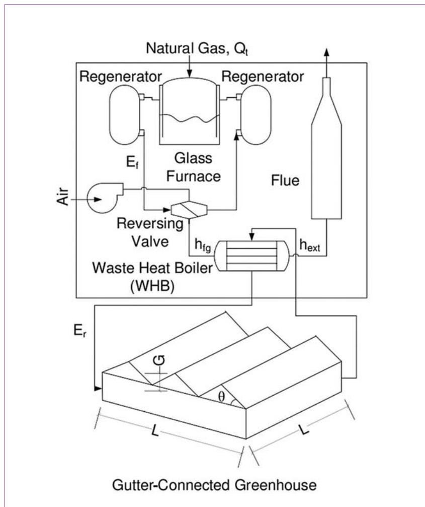
Figure 4. Detail of industrial symbiosis between glass manufacturing and a greenhouse complex showing system structure and energy flows.
