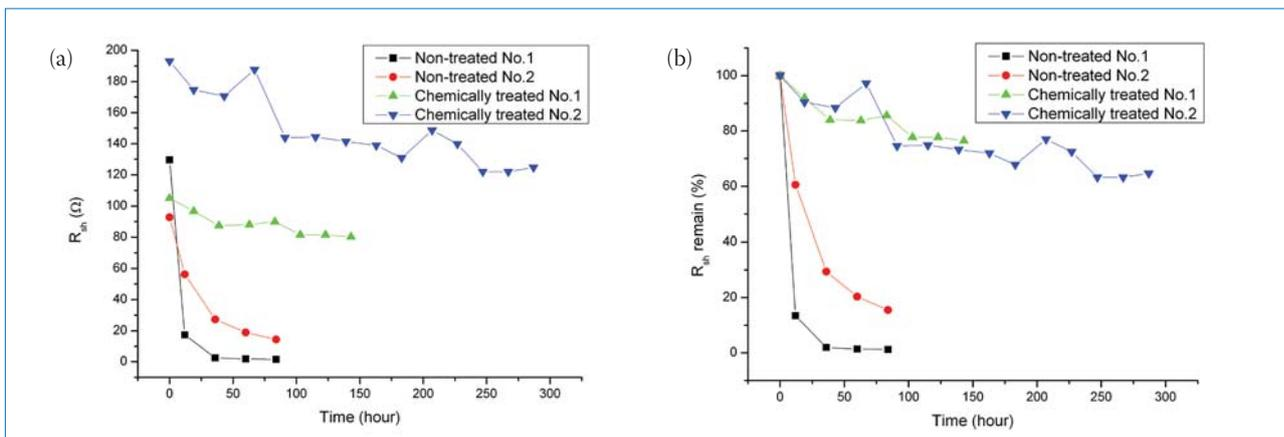
Figure 7. PID test results for normal and chemically treated modules: (a) change in  $R_{sh}$ , and (b) percentage  $R_{sh}$  remaining.
