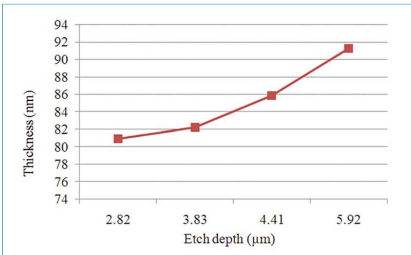
Figure 5. Antireflective film thicknesses for etch depths of 2.82μm, 3.83μm, 4.41μm and 5.92μm.
