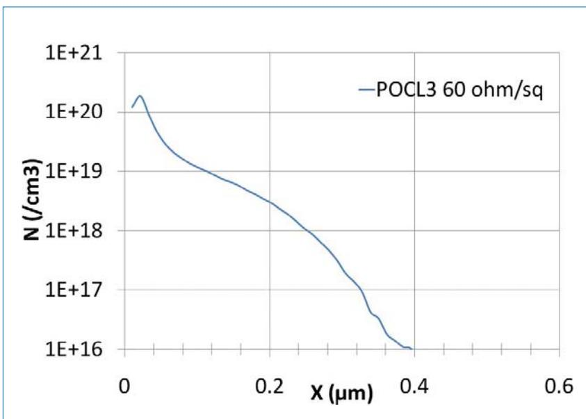
Figure 3. SIMS of a typical diffusion profile of a POCL<sub>3</sub> 60Ω/sq emitter.
