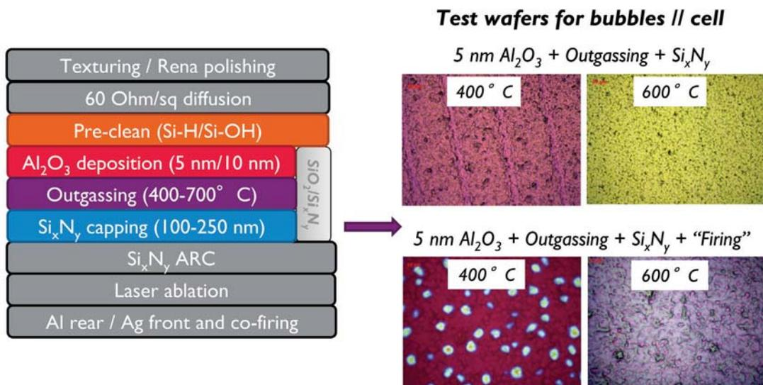
Figure 8. Blistering reduction with outgassing prior to Si<sub>3</sub>N<sub>4</sub> capping.
