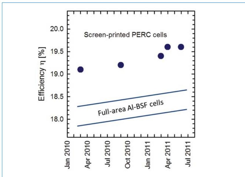
Figure 2. Recent record conversion efficiencies [14–19] of screen-printed rear-passivated PERC solar cells, applying large-area monocrystalline p-type silicon wafers. As a reference, typical conversion efficiencies [1] of industrially manufactured monocrystalline silicon solar cells, with a screen-printed full-area Al-BSF are also indicated.
