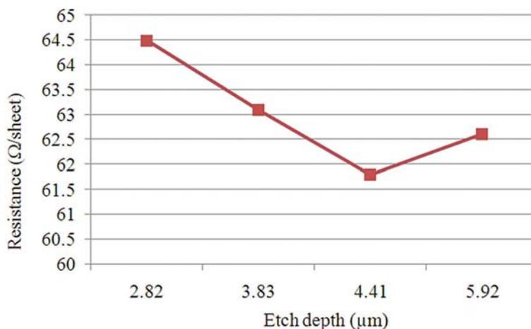
Figure 4. Sheet resistance for etch depths of 2.82µm, 3.83µm, 4.41µm and 5.92µm.
