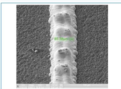
**OM Group Solar Chemicals' complete process for plated metal stack on fine-line printed Ag paste for c-Si cells**
