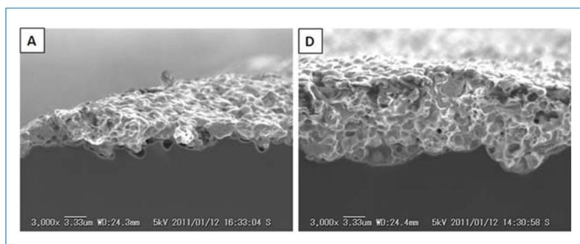
Figure 7. SEM images of bus-bar contact sections for different etch depths. Left: group A with etch depth 2.82μm. Right: group D with etch depth 5.92μm.
