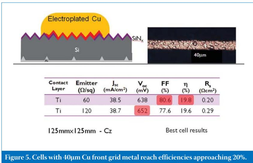
Figure 5. Cells with 40µm Cu front grid metal reach efficiencies approaching 20%.
