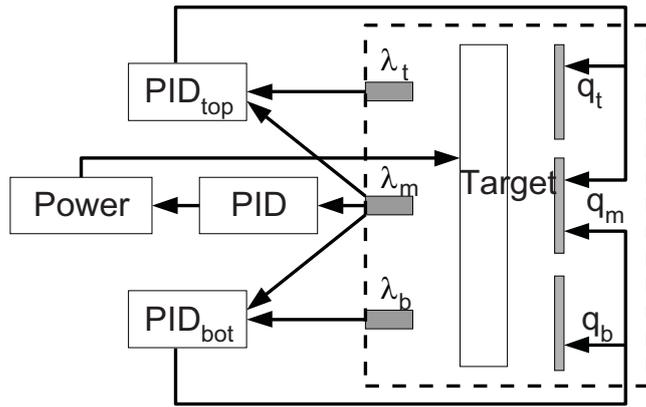
Figure 2. Principal setup of the symmetry control system used at Fraunhofer IST. Three  $\lambda$ -sensors are used to monitor oxygen partial pressure at different positions along the target. The measured values are used as input to a control loop for adjusting the flow of the threefold oxygen inlet.
