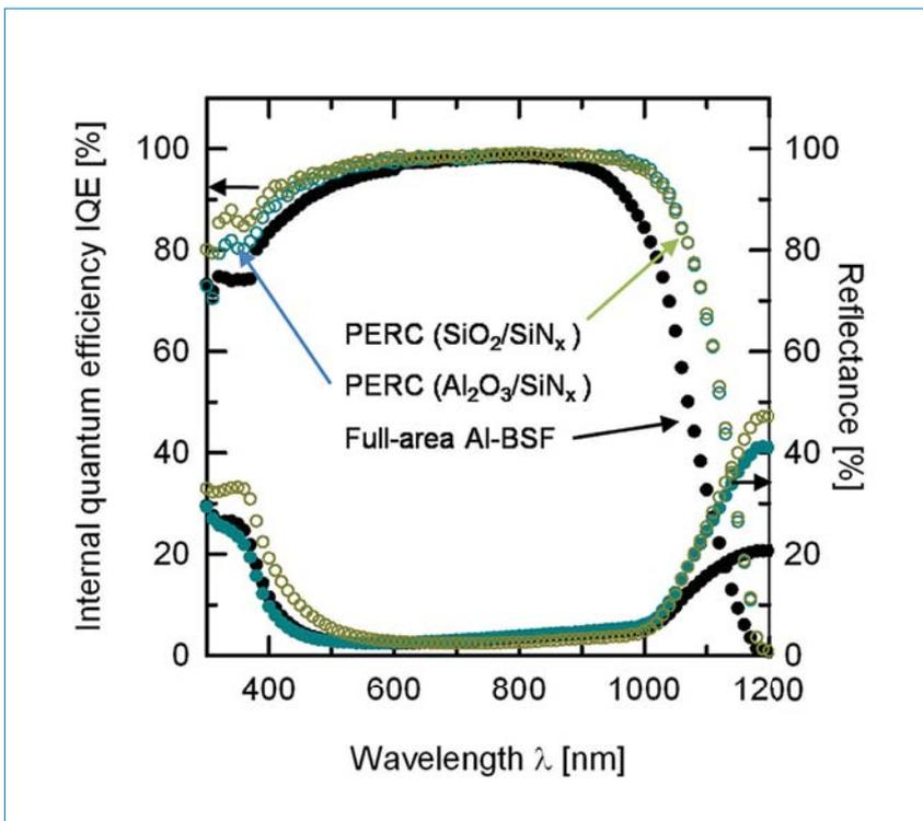
Figure 7. Comparison of IQE and reflectance between PERC solar cells with  $\text{Al}_2\text{O}_3/\text{SiN}_x$  (cell C in Table 1) and  $\text{SiO}_2/\text{SiN}_x$  (cell D) passivation stacks at the rear and a full-area Al-BSF reference cell ( $B_2$ ).
