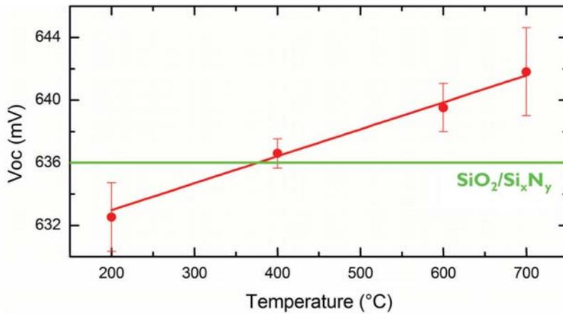
Figure 9. Increase in open-circuit voltage ( $V_{oc}$ ) as a function of outgassing temperature. Higher values than the reference  $\text{SiO}_2/\text{Si}_x\text{N}_y$  passivation stack are reached.
