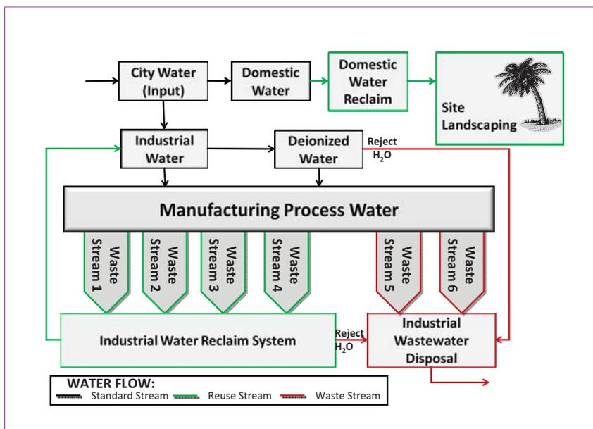
Figure 2. Water reuse scenario for a >120MW PV manufacturing facility.
