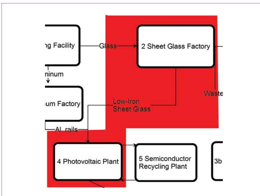
Figure 2. Detail of industrial symbiosis between PV and glass manufacturing.
