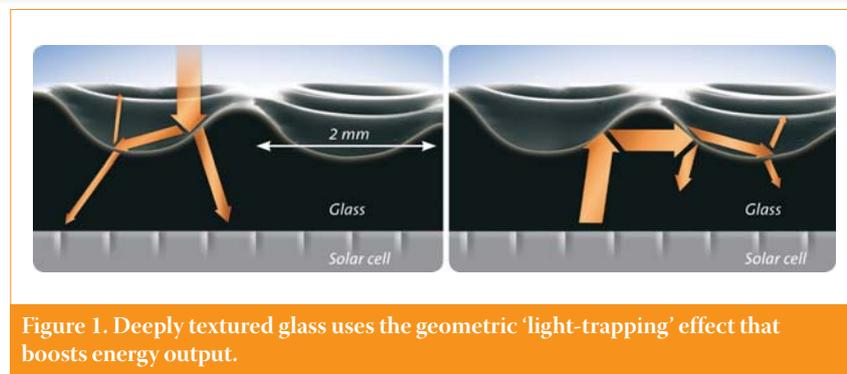
Figure 1. Deeply textured glass uses the geometric 'light-trapping' effect that boosts energy output.
