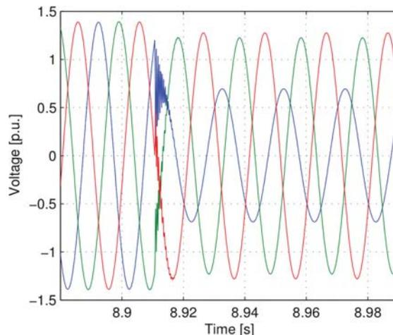
Figure 6. Measured voltages during unbalanced faults. Left: Dd MV/LV transformer. Right: Dy MV/LV transformer.
