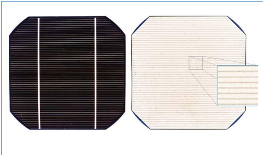
Figure 5. Photographs of the front and rear sides of a PERC solar cell with 19.4% conversion efficiency. Whereas the front side is very similar to a standard screen-printed solar cell, the rear side shows the dielectric passivation layer and the local line contacts.
