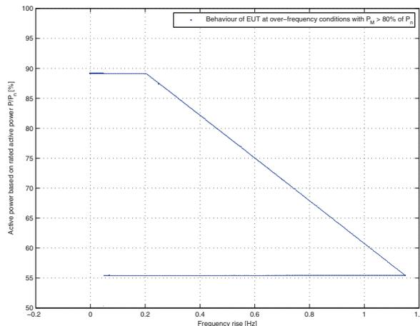
Figure 7. Measurement results for active power reduction corresponding to the over-frequency behaviour of the STP15000TL string inverter.
