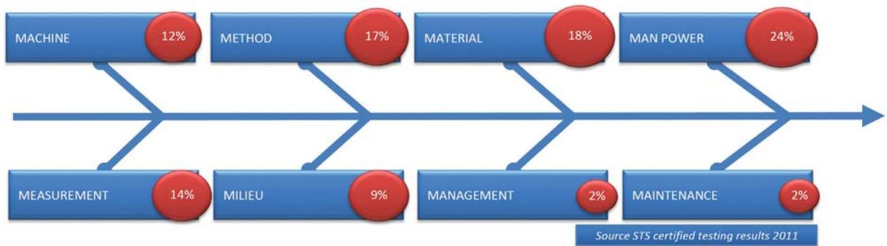
Figure 3. A breakdown analysis of the causes of failures (also known as 8M analysis) showing, in the form of a fishbone diagram, the distribution of the causes attributed to the defects detected during STS inspections and testing activities.
