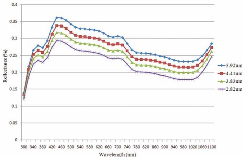
Figure 3. Surface reflectance at different wavelengths for etch depths of 2.82µm, 3.83µm, 4.41µm and 5.92µm.
