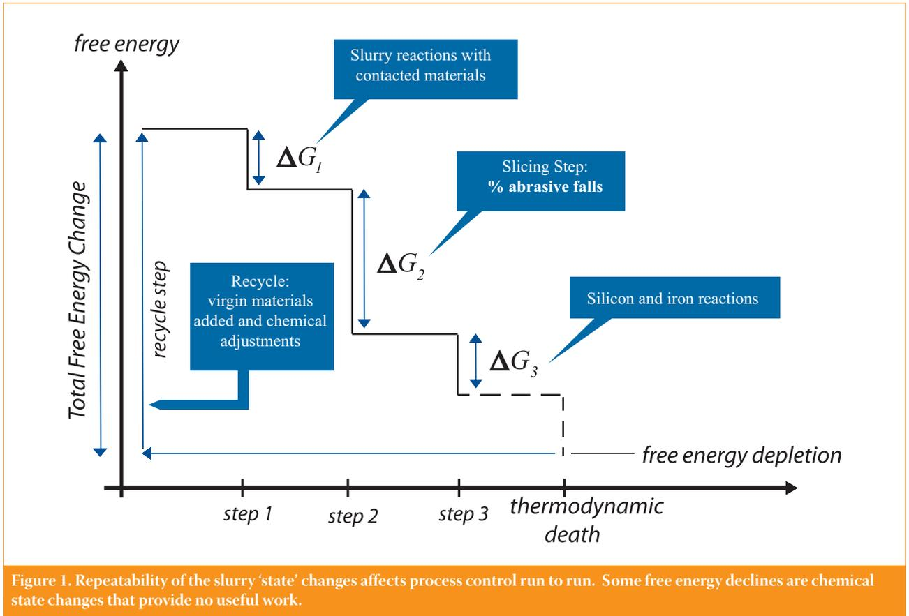
Figure 1. Repeatability of the slurry 'state' changes affects process control run to run. Some free energy declines are chemical state changes that provide no useful work.
