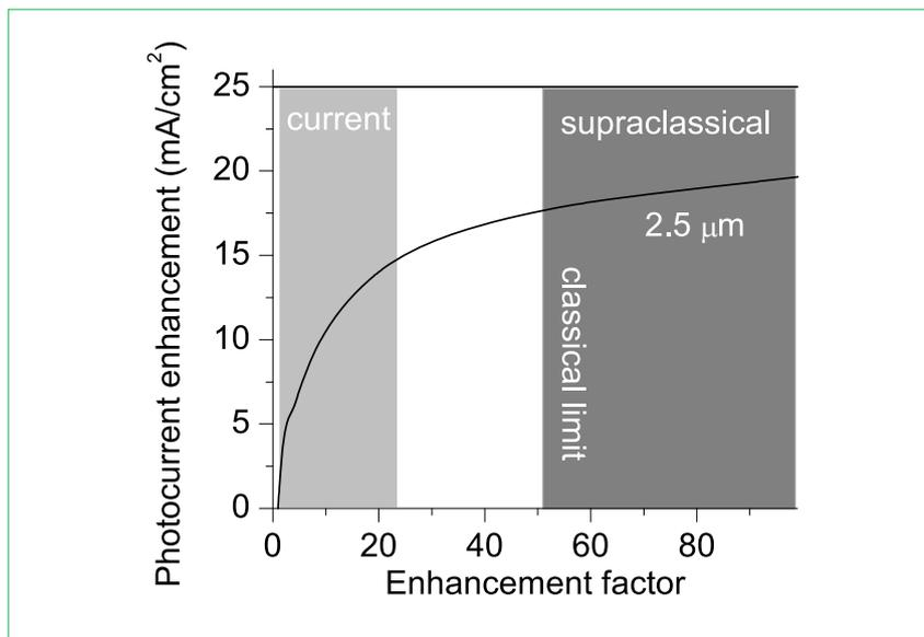
Figure 5. Enhancement in photocurrent with multiple reflections.
