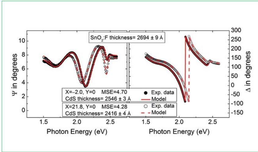
Figure 13. Experimental (points) and best-fit (lines) ( $\psi$ ,  $\Delta$ ) spectra at positions ( $X = -2.0$ ,  $Y = 0$ ) and ( $X = 21.8$ ,  $Y = 0$ ) in Fig. 12(a), showing the effect of the CdS thickness on the data and fits. The  $\text{SnO}_2\text{:F}$  thickness was almost the same for the two positions and within  $2694 \pm 9 \text{ \AA}$ . Confidence limits and mean square errors (MSEs) for the two best fits are also given.
