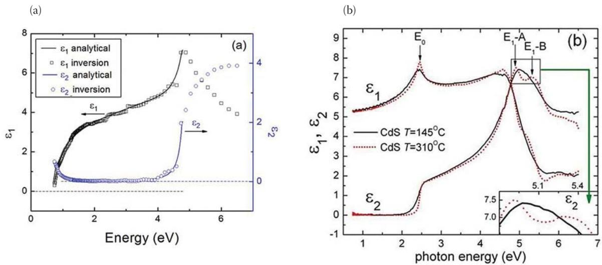
Figure 11. (a) Room temperature dielectric function of the topmost  $\text{SnO}_2\text{:F}$  layer of NSG-Pilkington TEC-15 glass; both methodologies of exact inversion (points) and analytical fitting below 4.8eV (lines) are shown and are in good agreement; (b) room temperature dielectric functions of two cadmium sulphide (CdS) thin films prepared by magnetron sputtering at substrate temperatures of 145°C and 310°C.
