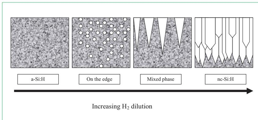
Figure 3. A schematic drawing of material structure changes with increasing hydrogen dilution.
