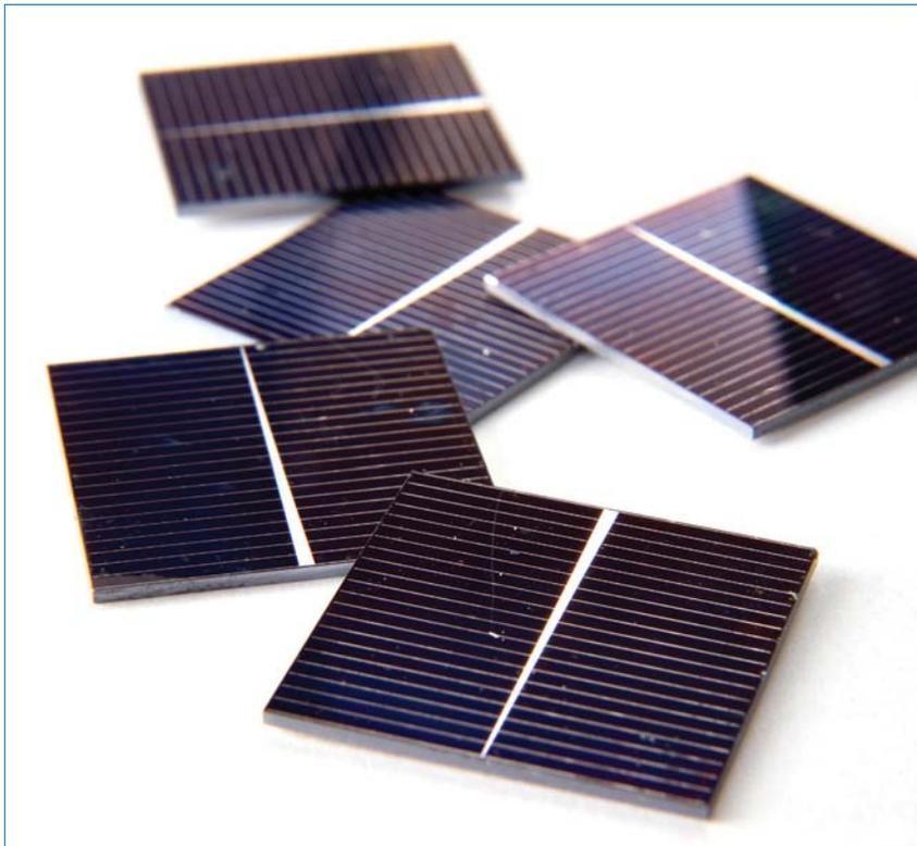
Figure 2. Imec's thin-film epitaxial Si solar cells – one of the pathways to working with very thin Si layers.
