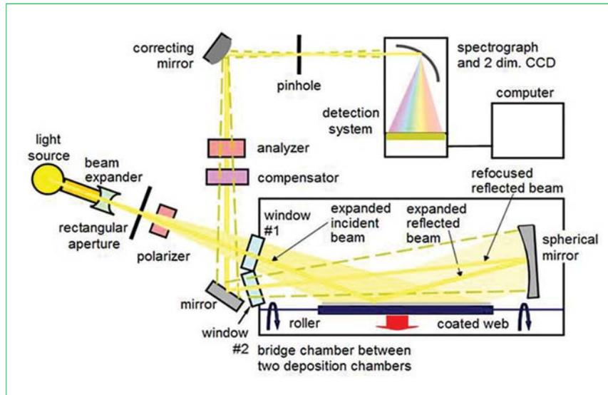
Figure 16. Simplified schematic of instrumentation for on-line SE imaging across the substrate width in conjunction with mapping along its length made possible by translation of the substrate on the production line. Although the design is shown for analysis of the coated substrate in roll-to-roll deposition, it can also be used in mapping moving glass panels.
