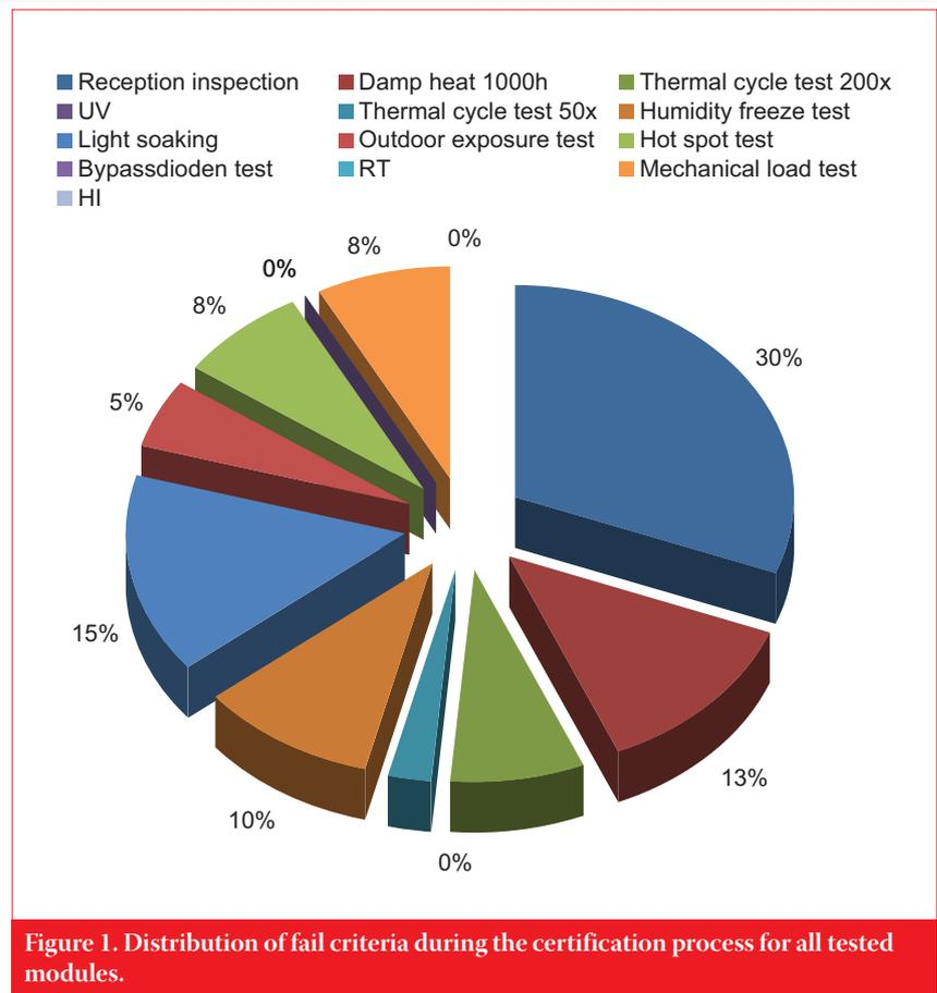
Figure 1. Distribution of fail criteria during the certification process for all tested modules.
