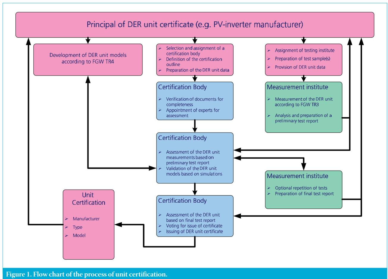
Figure 1. Flow chart of the process of unit certification.
