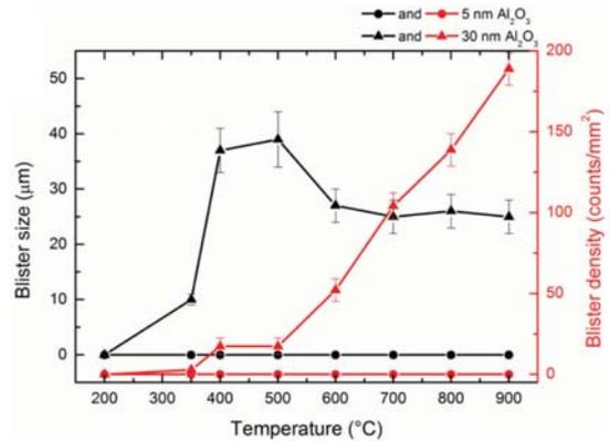
Figure 7. (a) Top-view SEM of a thick Al<sub>2</sub>O<sub>3</sub> layer showing blister formation; (b) blister density and size as a function of annealing temperature (350–900°C) for both a thin and a thick Al<sub>2</sub>O<sub>3</sub> layer.
