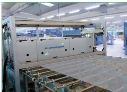
**dr. schwab IT's FPI solar metrology system enables fast full surface thickness evaluation of thin-film layers**
