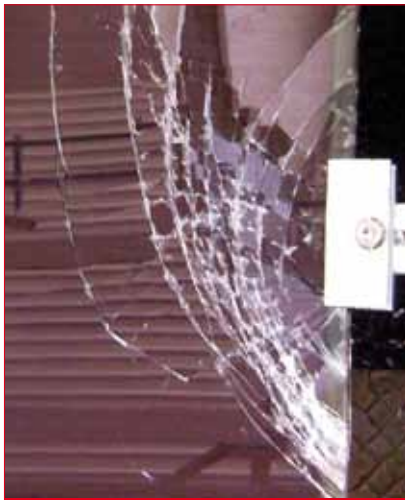
Figure 1. Breakage at 2,400 Pa: a-Si 1.4m 2 module with 2mm x 3mm glass.
