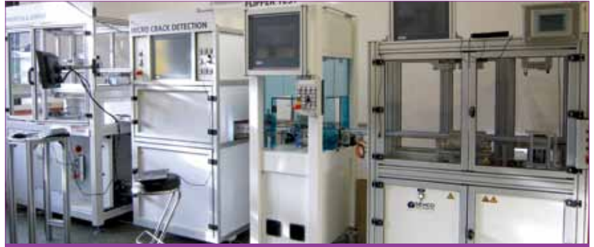
Figure 1. Automated test and demonstration platform for wafer handling experiments.
