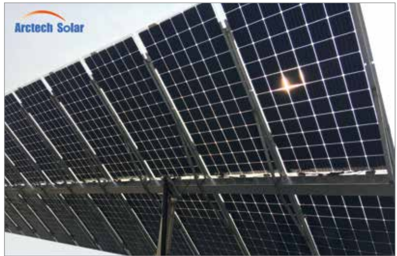
Figure 3. Independent horizontal single-axis tracker from Arctech Solar, designed for bifacial modules [145]. The modules are fixed using aluminium elements at the module edges, overlapping with the long purlins to avoid covering the back of the bifacial modules. Junction boxes at the module edges in such a system, as shown, can be integrated without shading caused by cables. (Source: Arctech Solar.)
