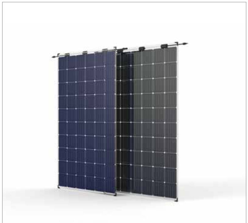
Figure 2. The DUOMAX Twin bifacial module from Trina, featuring a frameless glass/glass configuration with 60 monocrystalline cells (5BB) and p-type PERC cell technology; the reported bifaciality factor is greater than 70%. The module incorporates split junction boxes at the edge with three bypass diodes. The standard glass thickness is 2.5mm on both sides. The module efficiency ranges from 17.6 to 18.9% under STC conditions. (Source: Trina Solar.)
