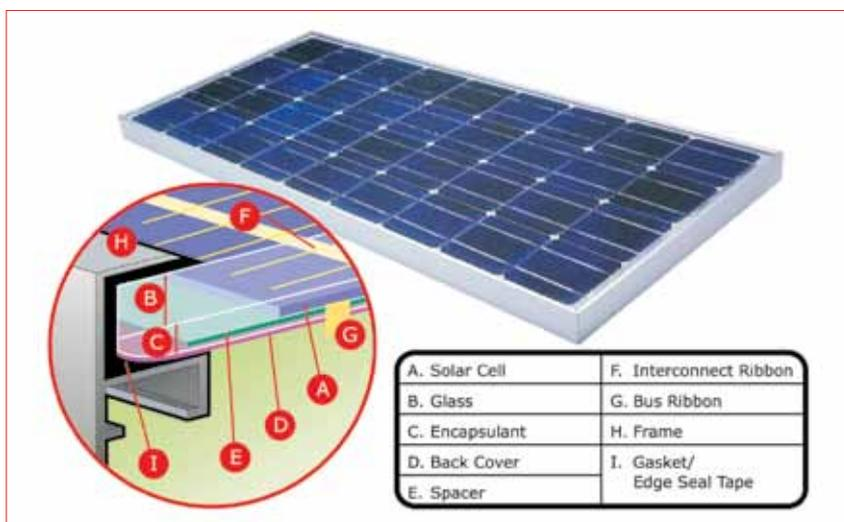
Figure 1. Cutaway view of a standard solar module.
