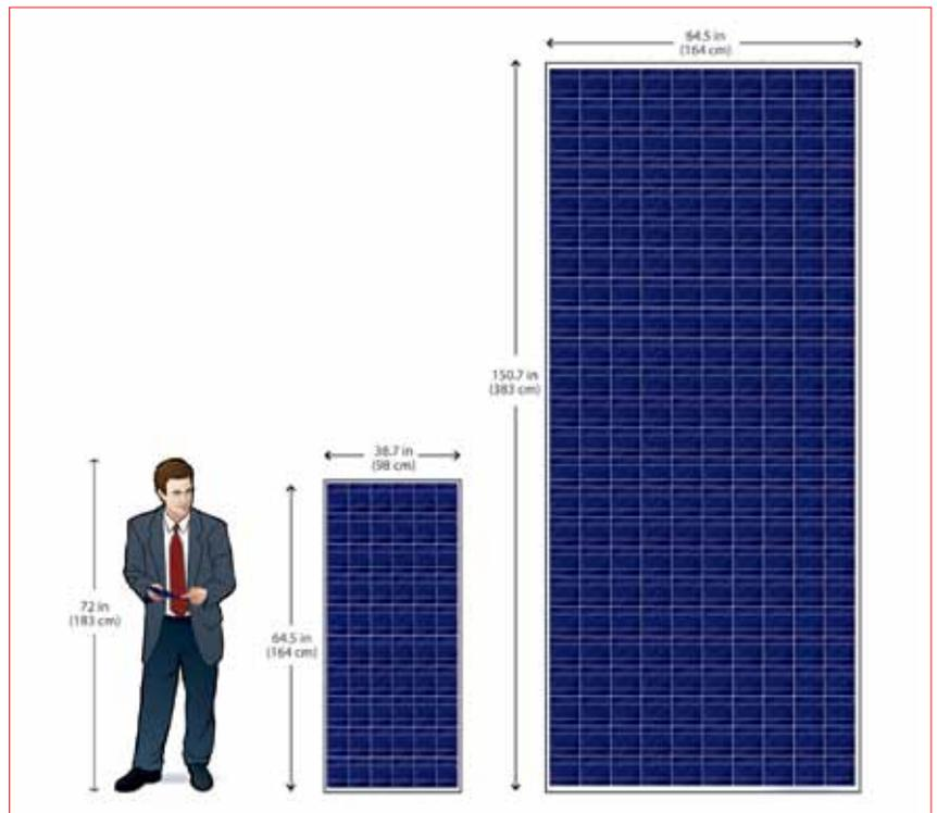
Figure 3. Comparison of standard (230W) and supersized (1kW) modules.
