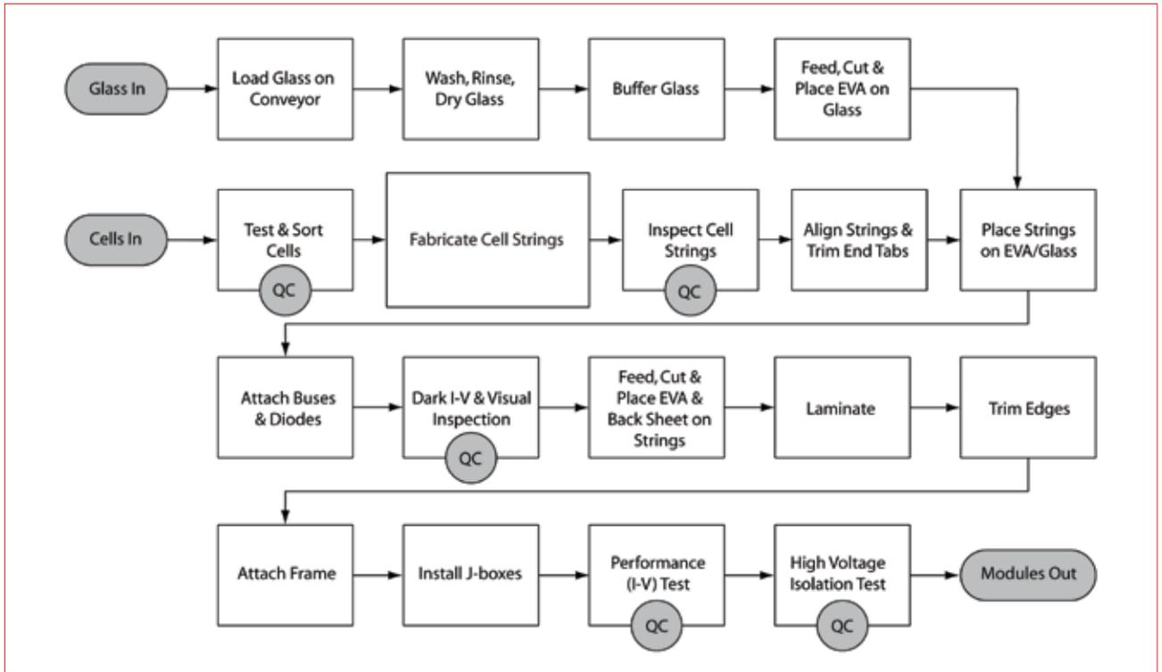
Figure 2. Standard solar module process sequence.
