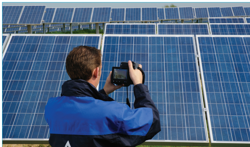
Figure 12. Infrared inspection to detect hot spots.
