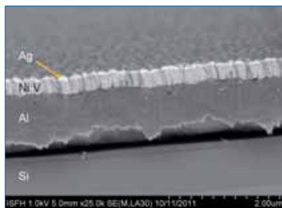
Figure 5. Cross-sectional SEM image of a metallization stack on a silicon wafer: 1 μm evaporated Al (dark grey with breaking edge in the bottom of the layer), 250 nm sputtered Ni:V (light grey) and 25 nm sputtered Ag (white).
