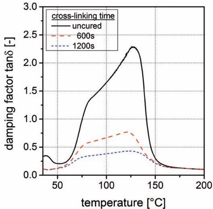
Figure 3. Temperature-dependent damping factor for uncured and partially cured EVA B film.
