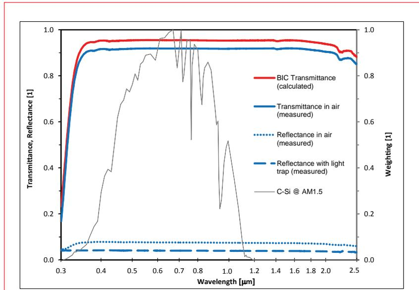
**Figure 7. Calculation of the BIC transmittance spectrum from three direct measurements: transmittance spectrum in air, reflectance in air, and reflectance with an optically coupled light trap. As indicated by the weighting spectrum (C-Si @ AM 1.5), it is mainly the transmittance in the range 0.4 $\mu\text{m}$  to 1 $\mu\text{m}$  that is of importance.**
