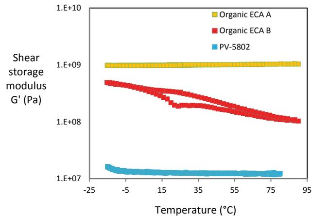
**Figure 3. Dynamic mechanical analysis of three cured ECAs. Organic ECA A is very stiff throughout the operating temperature range. Organic ECA B has a strongly varying modulus depending on the temperature. Dow Corning PV-5802 demonstrates a low modulus throughout the entire relevant temperature range.**
