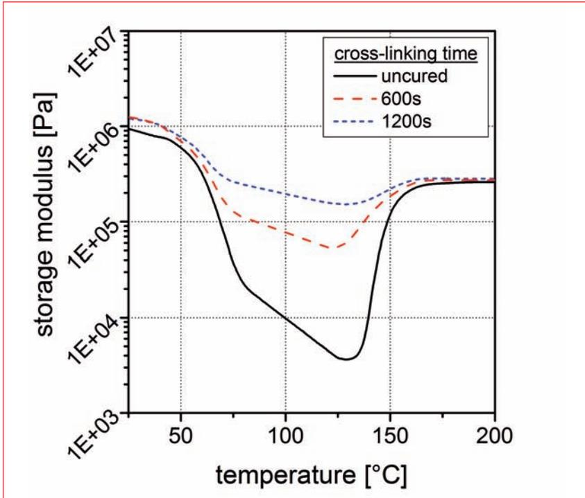
Figure 2. Temperature-dependent storage modulus for uncured and partially cured EVA B film.
