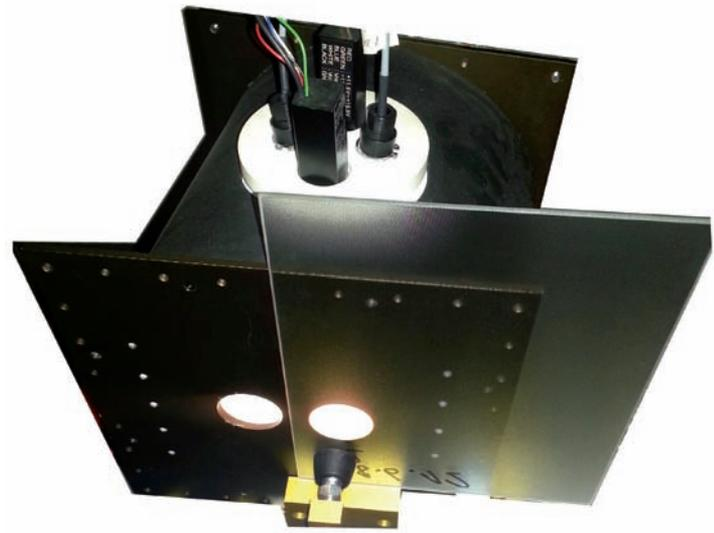
Figure 2. Sample glass in front of an integrating sphere at the SPF optical laboratory – the sphere is inside the black housing. During measurements, the sample glass covers one of the two sphere apertures. Four detectors with different wavelength sensitivities are fixed on the top of the sphere.
