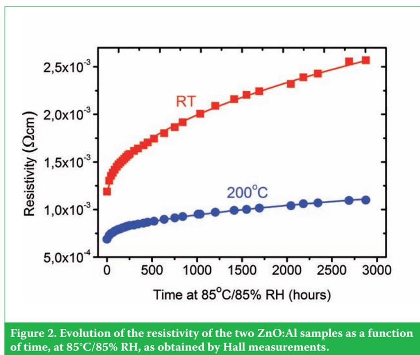
Figure 2. Evolution of the resistivity of the two ZnO:Al samples as a function of time, at 85°C/85% RH, as obtained by Hall measurements.
