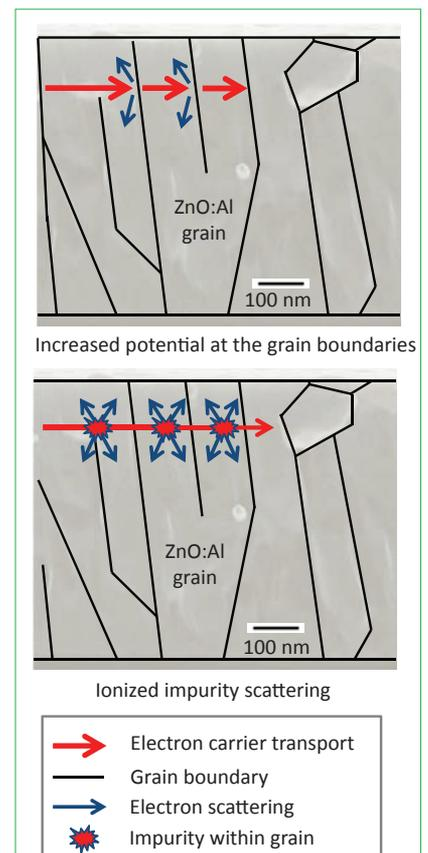
Figure 4. Possible scattering mechanisms in ZnO samples (based on Steinhauser et al. [10]).
