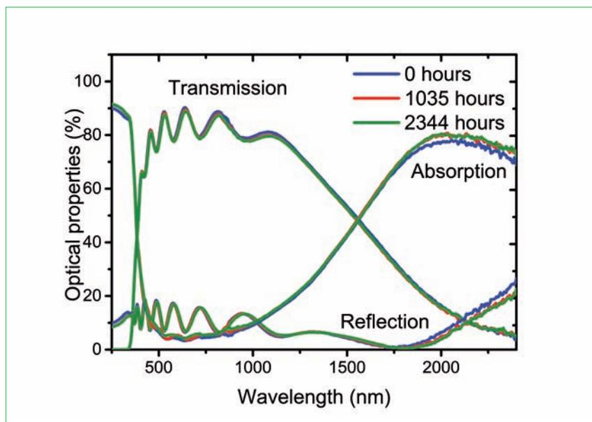
Figure 5. Evolution of the optical properties of the RT sample before and after exposure to 85°C/85% RH.
