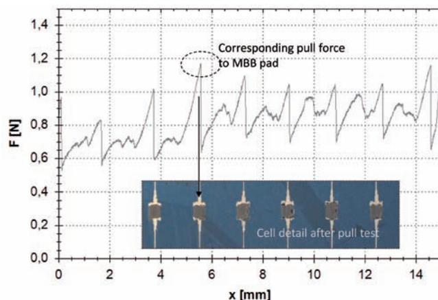
Figure 8. Typical force-pad sequence of the contact force measurements, showing that the wire had been soldered to every single pad.
