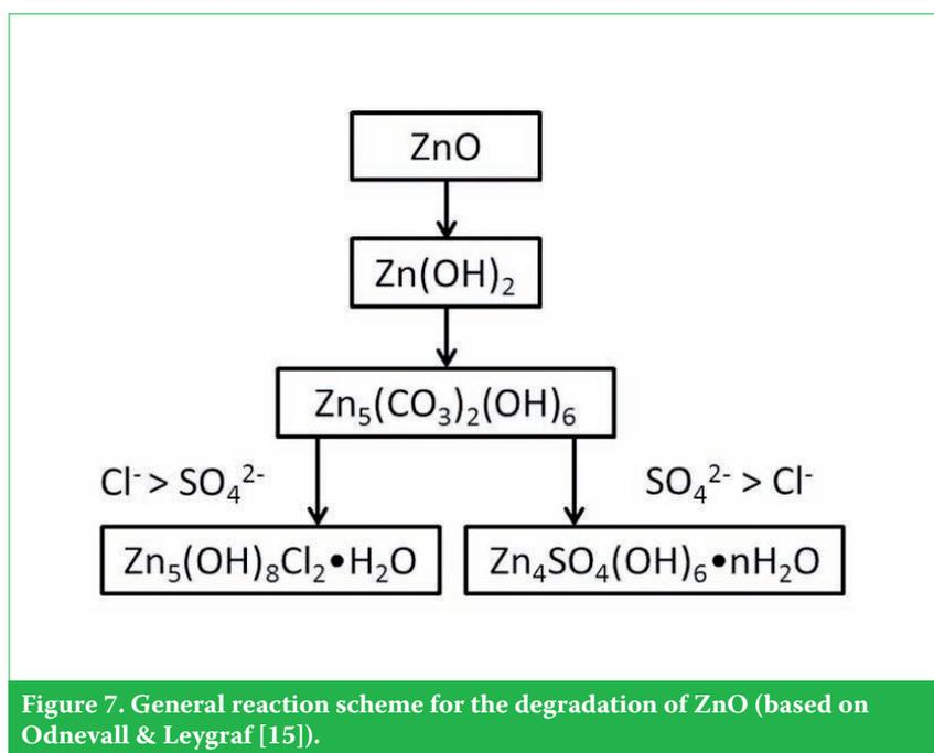
Figure 7. General reaction scheme for the degradation of ZnO (based on Odnevall & Leygraf [15]).
