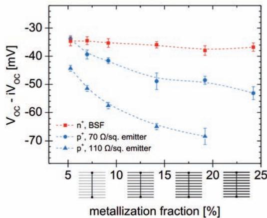
Figure 5. Net loss in cell  $V_{oc}$ , with respect to the implied  $V_{oc}$  value measured before metallization, as a function of screen-printed metal fraction on either a  $p^+$  emitter or an  $n^+$  BSF bifacial BiSoN cell.
