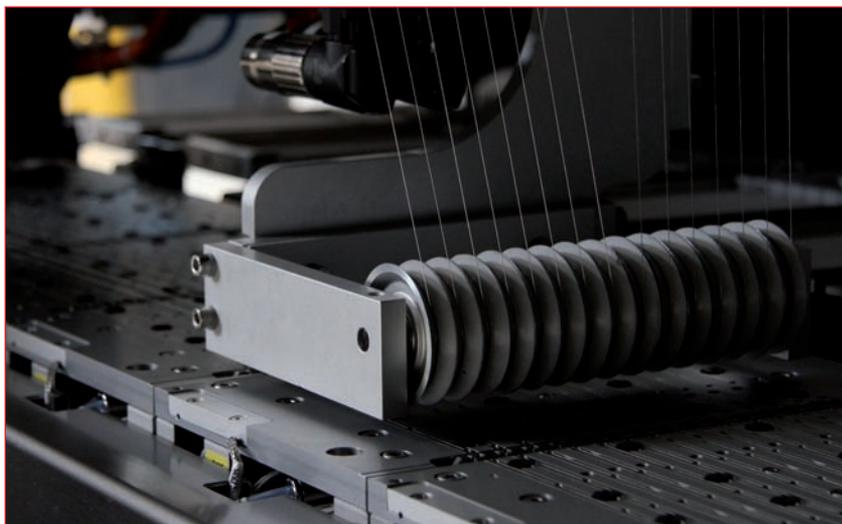
Figure 3. Multi-busbar connector: vacuum chuck used to align the 15 Cu wires on the solar cell.
