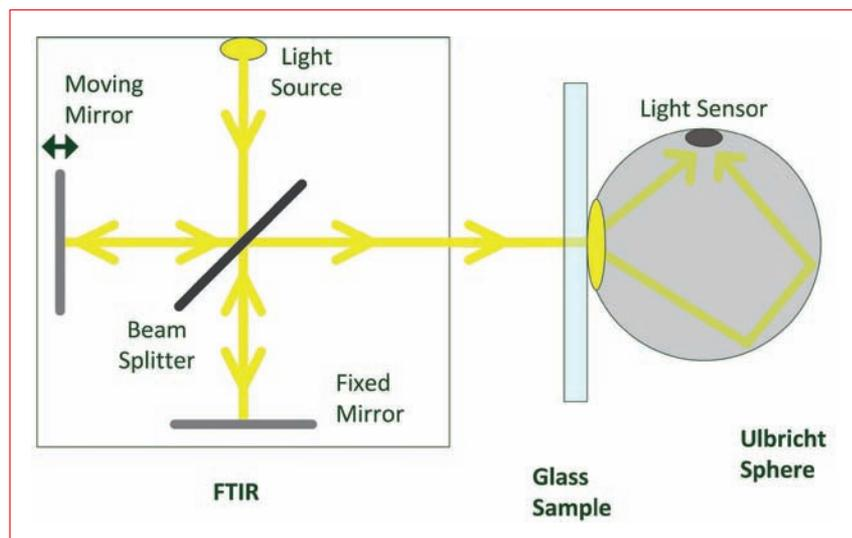
Figure 1. Measurement of direct/hemispherical transmittance using an integrating sphere. The diagram shows a Fourier transform spectrometer (FTIR), but other types of spectrometer can also be combined with integrating spheres.
