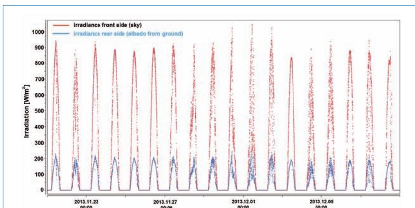
Figure 11. Outdoor measurements taken at the ISC Konstanz module test site: front-side (red) and rear-side (blue) irradiances measured on a bifacial module (20-degree fixed tilt) installed in the desert near El Gouna in Egypt.
