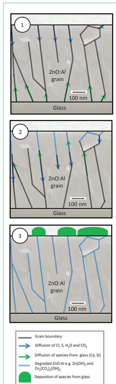
Figure 8. Proposed degradation mechanism for ZnO:Al layers.
