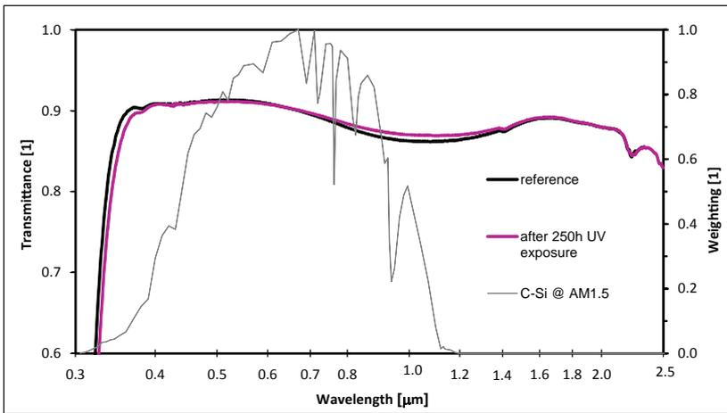
**Figure 12. Comparison of the conventional transmittance spectra of a solar glass with iron contamination (no. 2) before and after UV exposure. The change in spectral transmittance is caused by photo-oxidation of  $Fe^{2+}$  to  $Fe^{3+}$  and leads to a slight increase in the transmissivity.**
