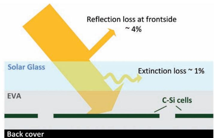
Figure 4. Simplified model of the optical losses caused by the glass in a PV module set-up.
