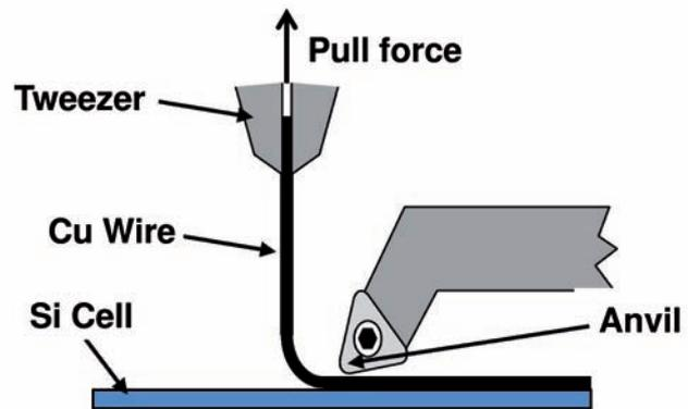
Figure 7. Test set-up for the mechanical pull tests.
