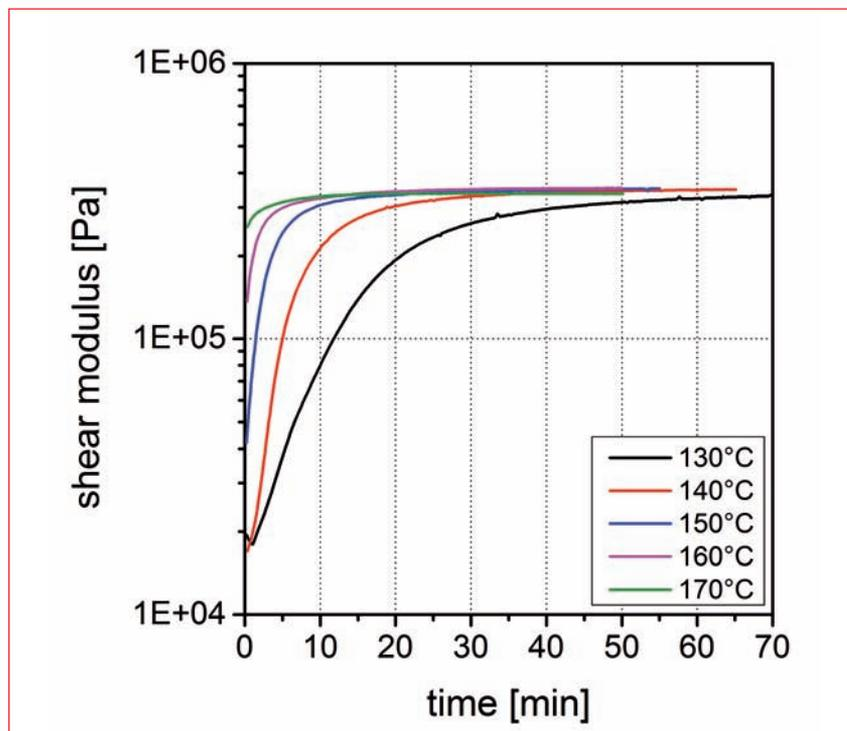
Figure 6. Storage modulus of EVA B as a function of time at constant temperatures between 130 and 170°C.
