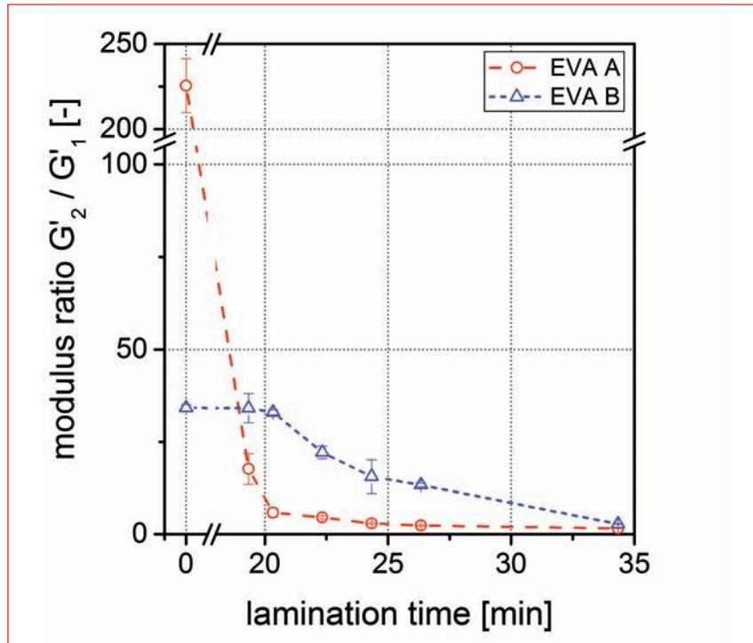
Figure 5. Modulus ratio  $G'_2/G'_1$  as a function of lamination time.
