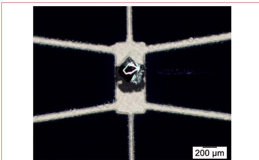
**Figure 12. Detailed microscopy image of the fracture mode after the pull test, with conchoidal fracturing of silicon within the pad area.**
