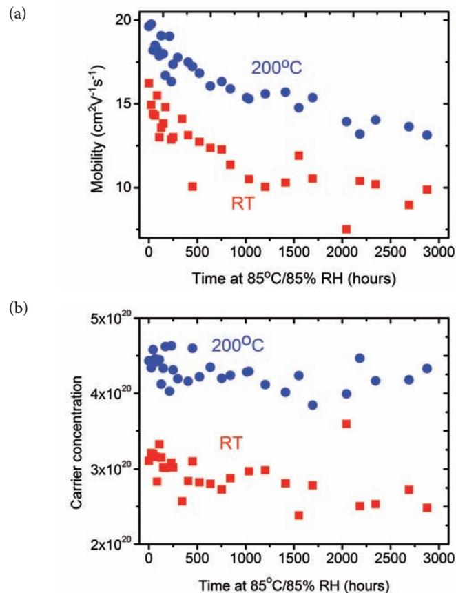
Figure 3. Hall mobility (a) and carrier concentration (b) of ZnO:Al as a function of time, at 85°C/85% RH.
