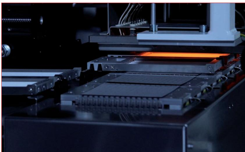
Figure 4. Multi-busbar connector: cell vacuum chucks and the IR soldering unit for the soldering process.
