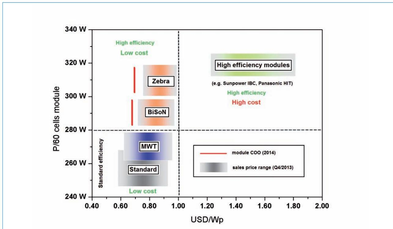
**Figure 10. Efficiency (expressed as the Pmpp of a 60-cell module, assuming 6" cells), COO and possible sales price ranges (US\$/Wp) for BiSoN and ZEBRA modules compared with various PV technologies currently available on the market.**
