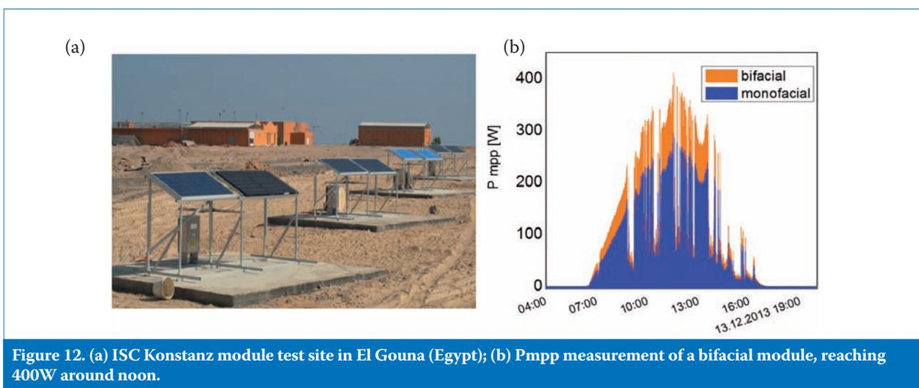
Figure 12. (a) ISC Konstanz module test site in El Gouna (Egypt); (b) Pmpp measurement of a bifacial module, reaching 400W around noon.
