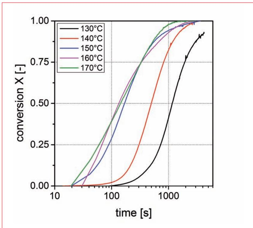
Figure 7. Conversion rate of EVA B as a function of temperature.
