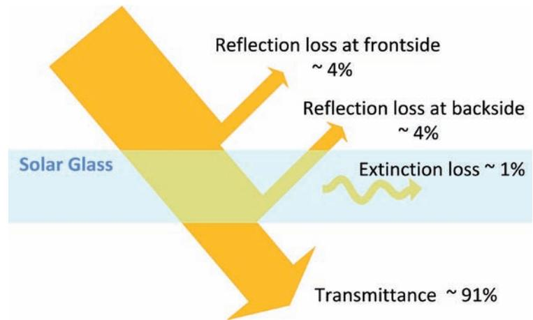
Figure 3. Optical losses of solar glass in an air–glass–air set-up.
