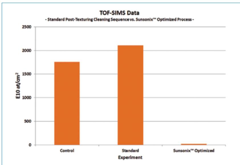
Figure 8. Comparison of standard post-texturing cleaning sequence to best process sequence (Test 1); TOF-SIMS results for Cu.
