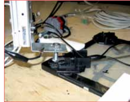
Figure 11. View of fatigue tester with junction box.
