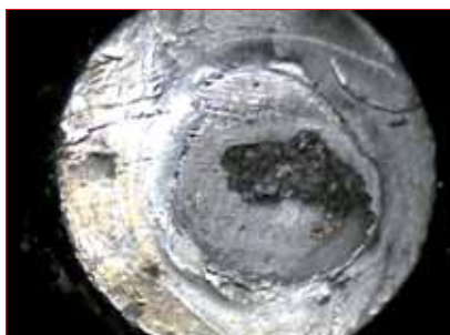
Figure 4. View of the junction-box pin following the first occurrence of a failure in thermal cycling.
