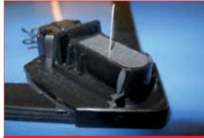
Figure 10. Coupon prepared to allow busbar deflection measurement as a function of quasi-steady state temperature.
