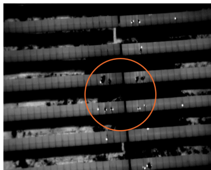
Figure 3. Vegetation over the modules detected with aerial inspections applying two different techniques: aIRT (left) and aerial visual inspection (right)
