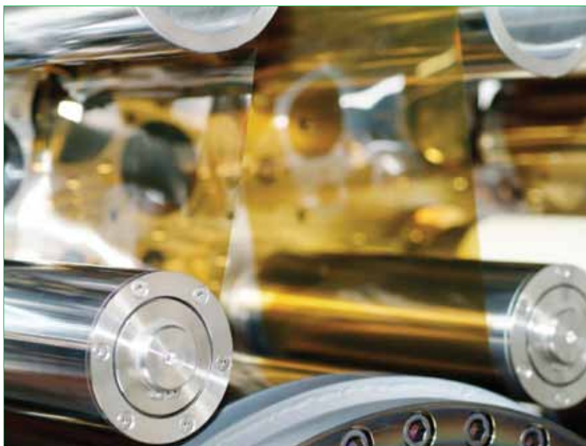
Figure 2. Solarion's low-cost roll-to-roll manufacturing technology.
