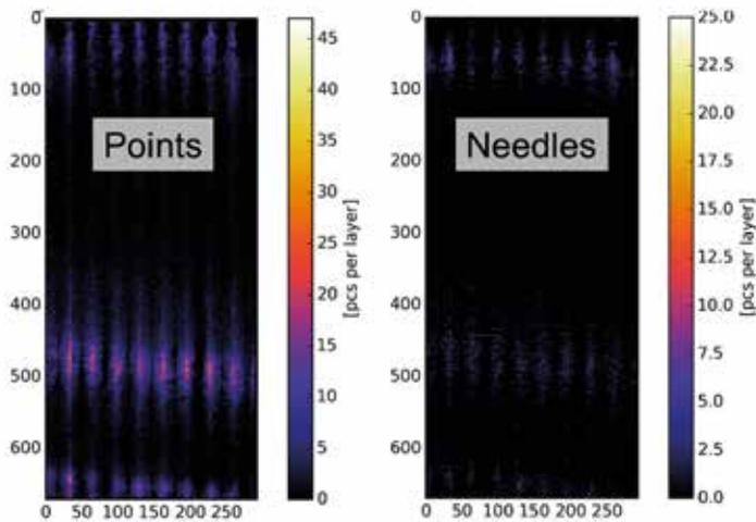
Figure 12. Bands of point- and needle-like defects detected by high-resolution IR transmission.
