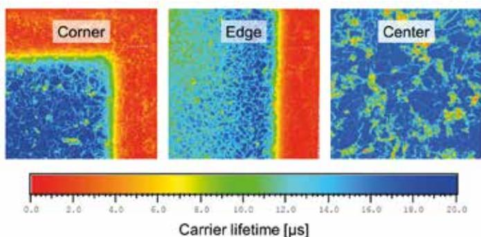
Figure 6. Carrier lifetime mappings of the bottom slabs prove the ingot position of the bricks.
