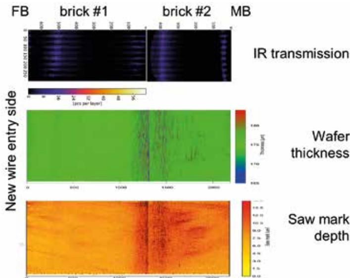
Figure 13. Correlation of precipitate bands with wafer thickness and saw mark depth in the second configuration.
