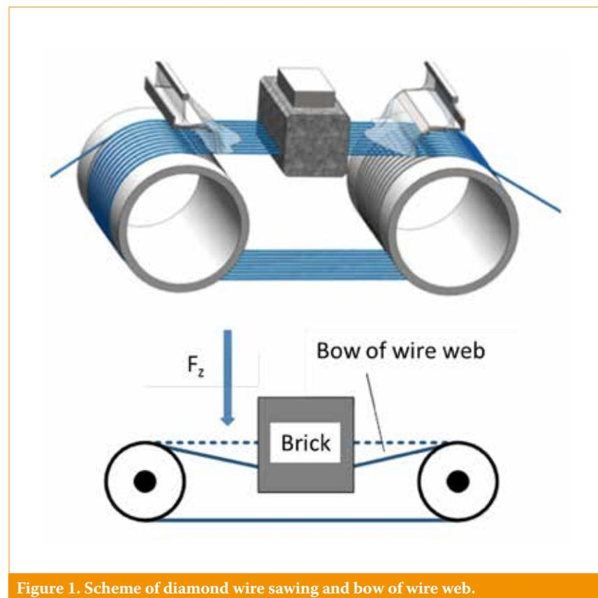
Figure 1. Scheme of diamond wire sawing and bow of wire web.
