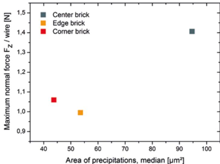
Figure 11. Correlation of  $F_z$  and the median precipitate area in the bottom and top slabs from the different HPM-Si bricks.
