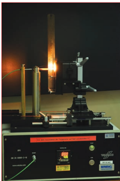
Figure 2. Glow-wire test: test for resistance to ignition.
