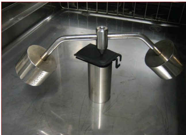
Figure 1. Ball pressure test: material test for resistance to heat.
