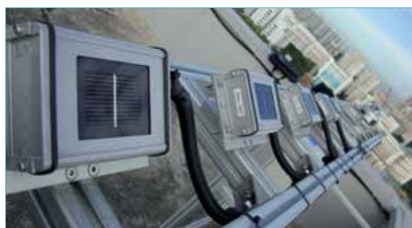
▼ Figure 4. The irradiance measurement station located on the roof at the Solar Energy Research Institute of Singapore (SERIS).
