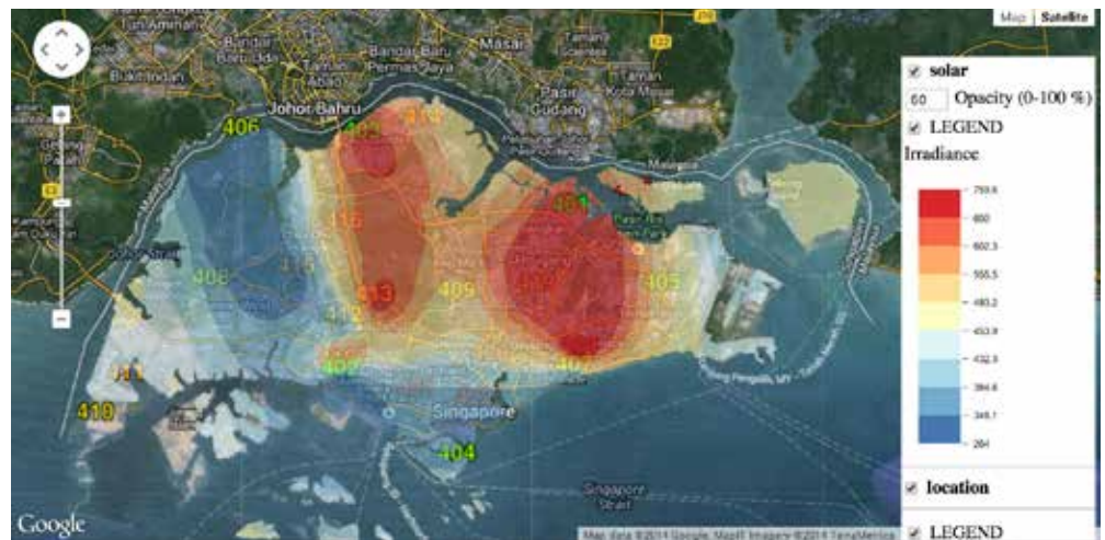
Figure 8. An interactive tool developed by SERIS, showing a live irradiance map taken at 12:00 noon on 1 February, 2014. Locations of the 25 irradiance measuring stations (numbered 401–425) in Singapore are shown. (Map: Google Maps, retrieved 1 February, 2014.)
