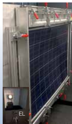
During 5400 Pa load (vacuum)
