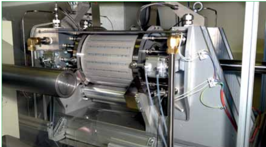
Figure 8. R2R tool for spatial ALD on 30cm-wide foils.
