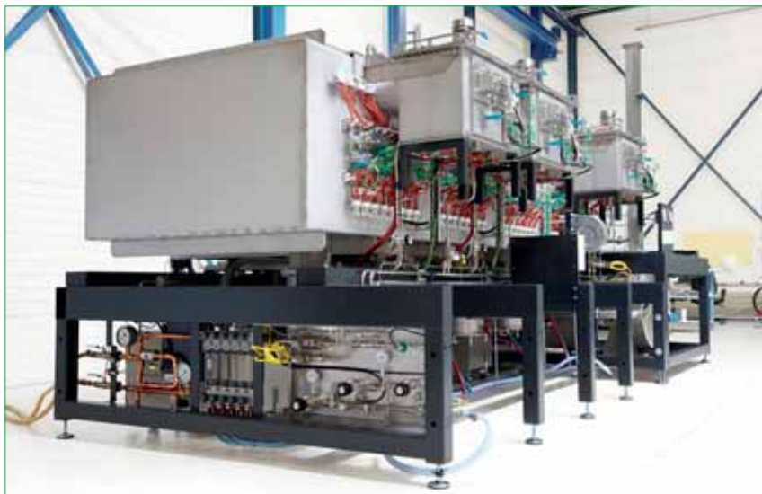
Figure 2. The R&D selenization tool built by Smit Ovens to facilitate process development at Solliance. One-to-one translation of the set-up to a full-scale production line is possible.
