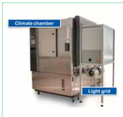
Figure 10. Hybrid degradation set-up, allowing exposure to illumination, elevated temperature and humidity.
