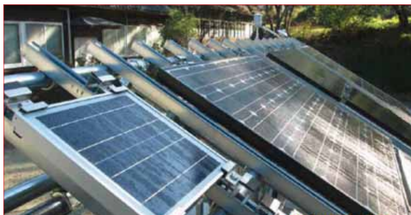
Figure 2. Morning dew responsible for the leakage current peak in the morning [4].
