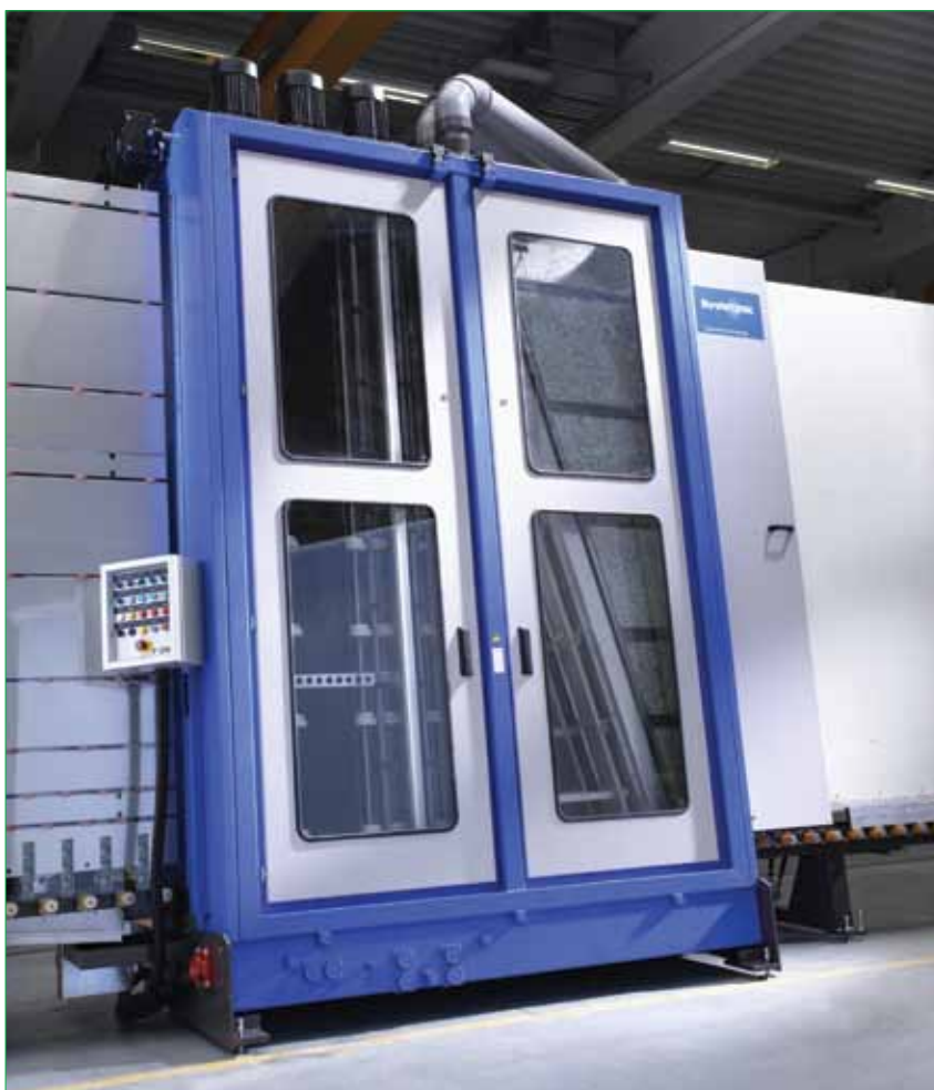
Figure 2. Vertical setup reduces footprint, avoids sag, and employs gravity for rinsing.
