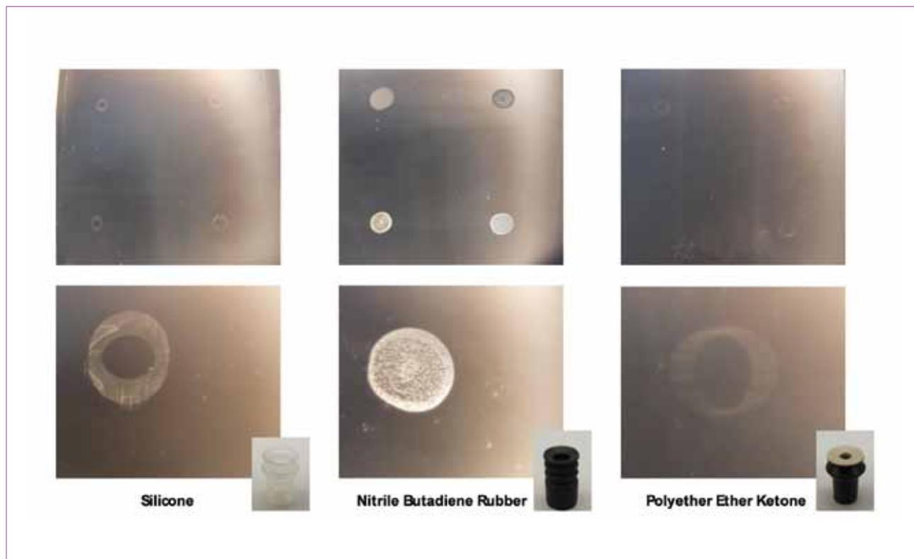
Figure 2. Visible imprints of different suction cup materials produced on as-cut wafers.
