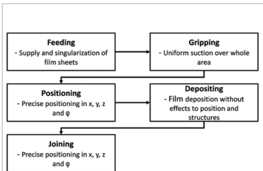
Figure 6. Handling steps for SMARTLAM foil handling.
