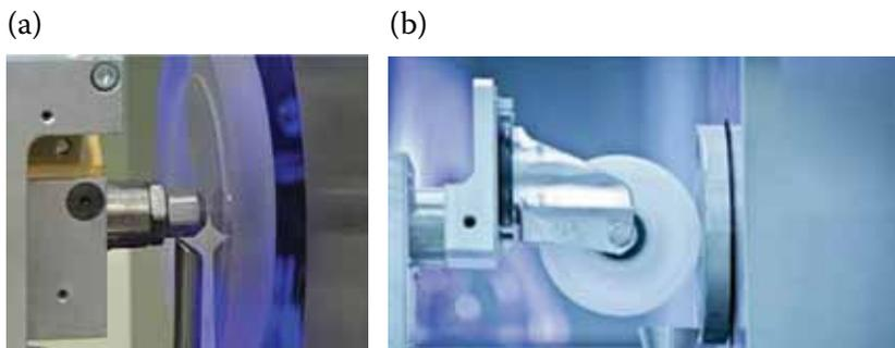
Figure 3. (a) Ball-disk test to simulate sliding friction; (b) roll-disk test to simulate rolling friction.
