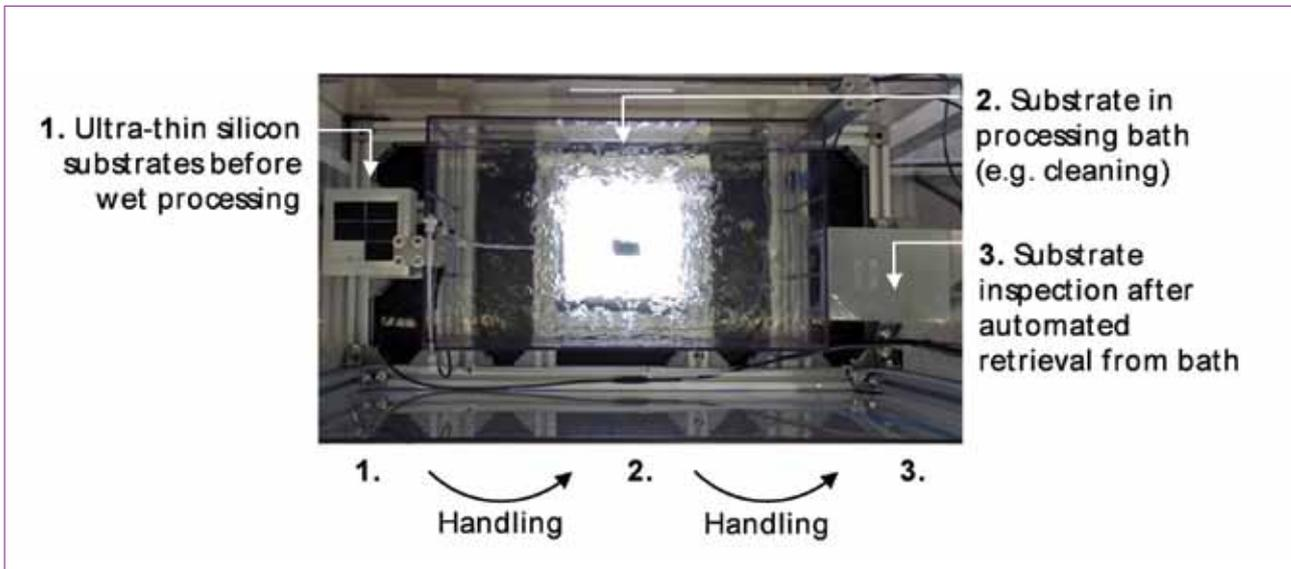
**Figure 8.** Top view of the test equipment for the automated handling of ultrathin substrates within wet processes. The correlation is determined between the achievable accuracy of substrate detection and a reliable, gentle gripping for retrieving the ultrathin substrate from the cleaning bath.
