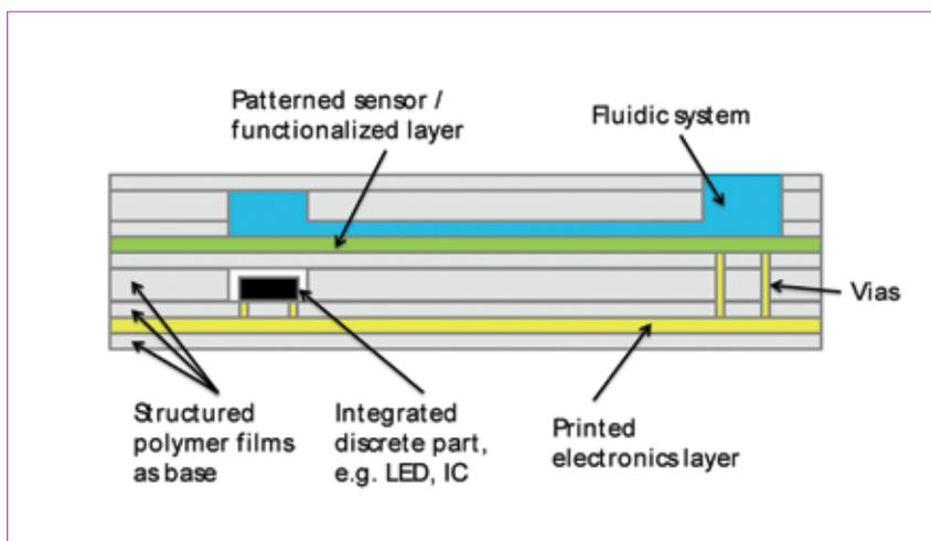
Figure 5. Example of a complex layer-based component.
