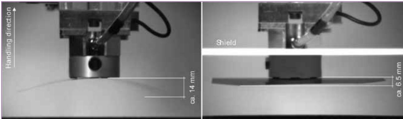
**Figure 1. Deformation of thinned 125mm × 125mm ultrathin wafers during high-speed handling with a Bernoulli gripper (vertical acceleration 25m/s<sup>2</sup>, travel velocity 3m/s). Aerodynamic issues become a more important factor in meeting future production throughput requirements.**
