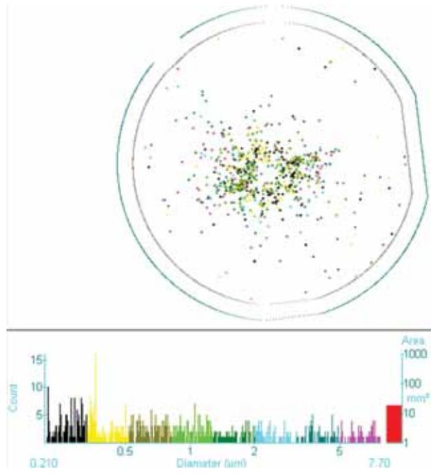
Figure 4. (a) Set-up of the ISO class 1 cleanroom handling experiment with a Bernoulli gripper above a clean and polished 4" silicon wafer. (b) Surface inspection result of one handled wafer after seven gripping cycles – 1.5 bar supply pressure, 7-sec activated gripping each cycle. Gain value 0.21–7.7µm: twenty times more particles.
