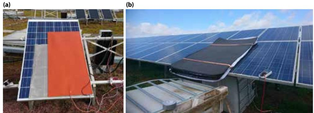
**Figure 2. (a) Grounding metal sheet (silver) and heating pad (orange) attached to a freestanding module on a test field; (b) the same set-up, covered by the heat-insulating blanket (black), deployed in a large-scale PV power plant**
