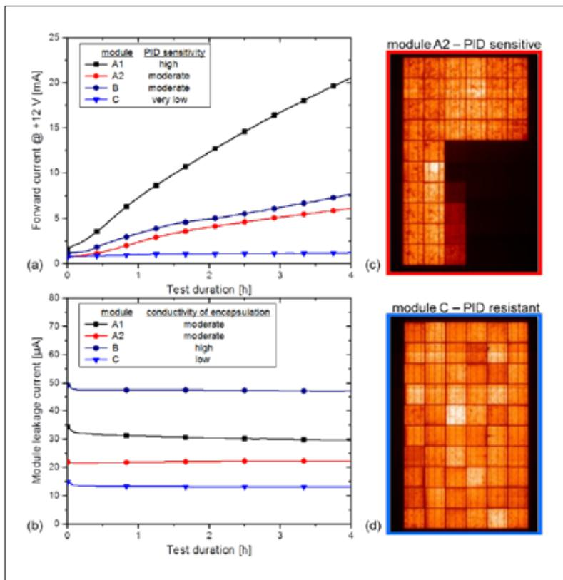
Figure 4. (a) Forward current and (b) measured leakage current for four different modules subjected to the outdoor PID test procedure; EL images acquired after the PID test for (c) the PID-susceptible module A2, and for (d) the PID-resistant module C
