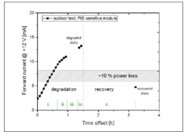
Figure 5. Forward current and measured leakage current of a module undergoing the PID test procedure in real outdoor conditions at a PV power plant
