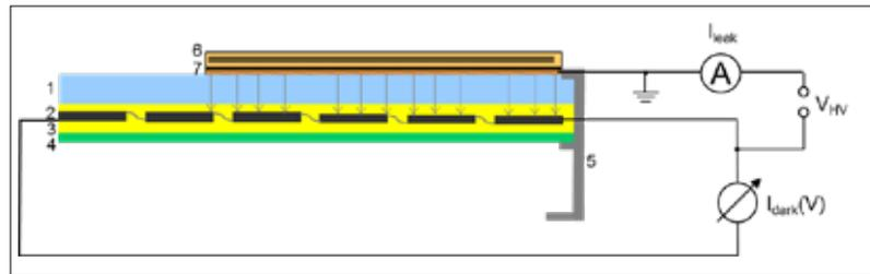
**Figure 1. Wiring scheme for the PID test (1: module cover glass, 2: cells, 3: encapsulation polymer, 4: backsheet, 5: module frame, 6: heating pad, 7: metal sheet for grounding)**
