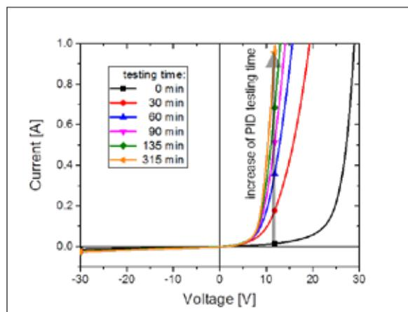
**Figure 3. Dark  $I$ - $V$  curves, acquired in situ, of a 60-cell module ( $V_{oc} = 36V$ ) when 24 cells were subjected to a PID stress of  $-1,000V$  at 85°C, showing the evolution of PID with time**
