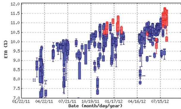
Figure 3. Box plot with a timeline of a-Si/ $\mu$ c-Si (initial) tandem cell efficiency values realized at PVcomB for different TCO substrates: FTO (blue) and AZO (red). A two-month downtime for maintenance and hardware modifications can be seen in spring 2012.
