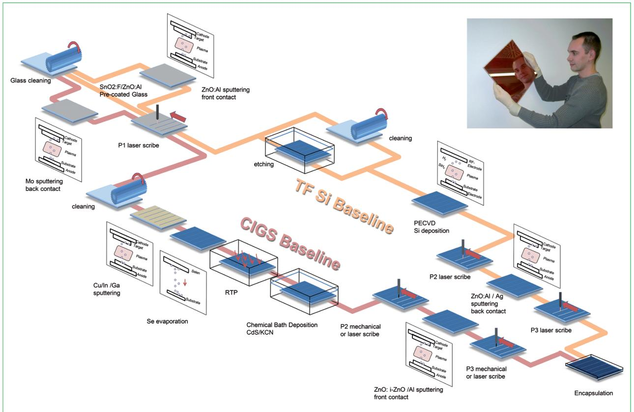
Figure 1. Schematic representation of the two 30×30cm<sup>2</sup> reference lines for TF Si (a-Si/μc-Si) and CIGS modules.
