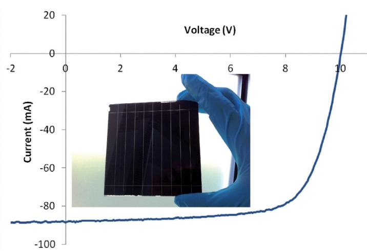
Figure 4. *I-V* characteristics of an a-Si/ $\mu$ c-Si mini-module (seven cells, 56cm<sup>2</sup> aperture area) from the PVcomB baseline, with 11.3% (initial) efficiency.
