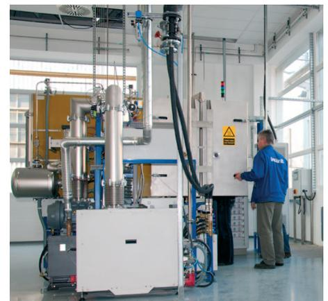
PE-CVD reactor for thin layers.
