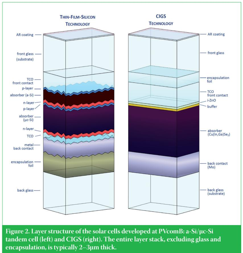
Figure 2. Layer structure of the solar cells developed at PVcomB: a-Si/μc-Si tandem cell (left) and CIGS (right). The entire layer stack, excluding glass and encapsulation, is typically 2–3μm thick.
