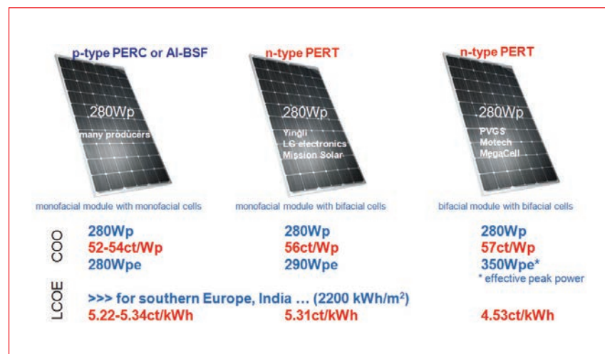
Figure 2. COO and LCOE for different Cz-Si module technologies. (For the bifacial module, a bifacial gain of 20% was assumed.)
