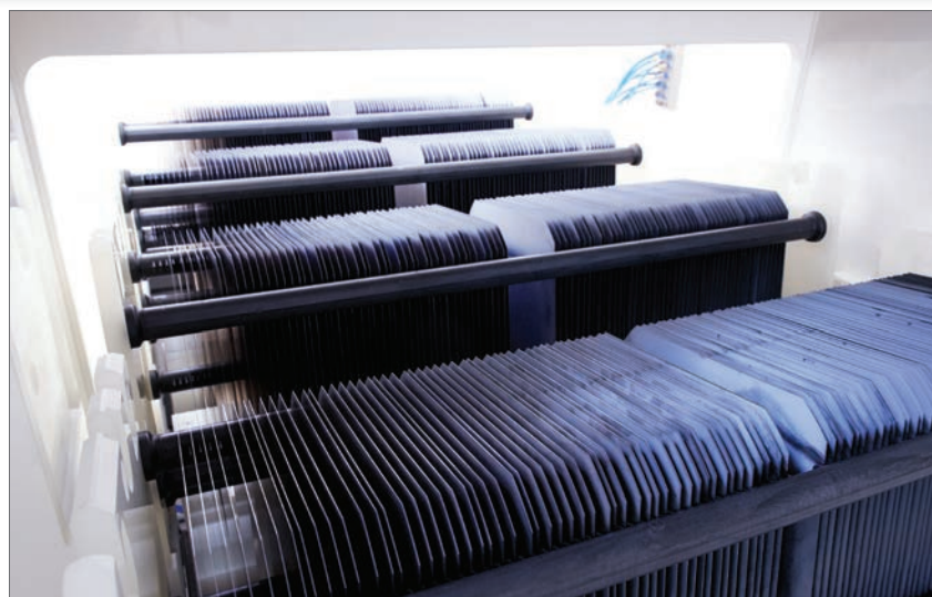
Figure 1. BiSon solar cell production: low-cost manufacture of high-efficiency n-type bifacial monocrystalline silicon solar cells.
