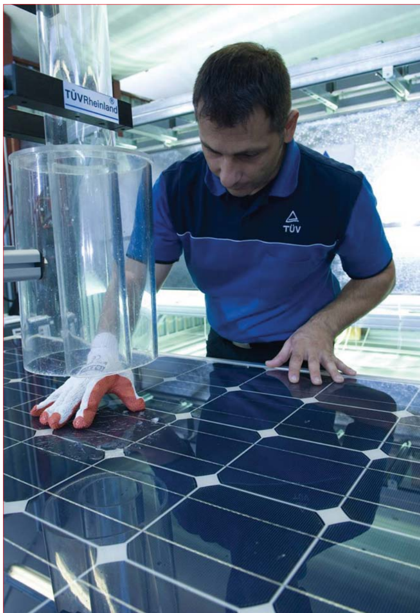
Figure 1. Module testing at TÜV Rheinland's PV laboratory in Cologne, Germany.
