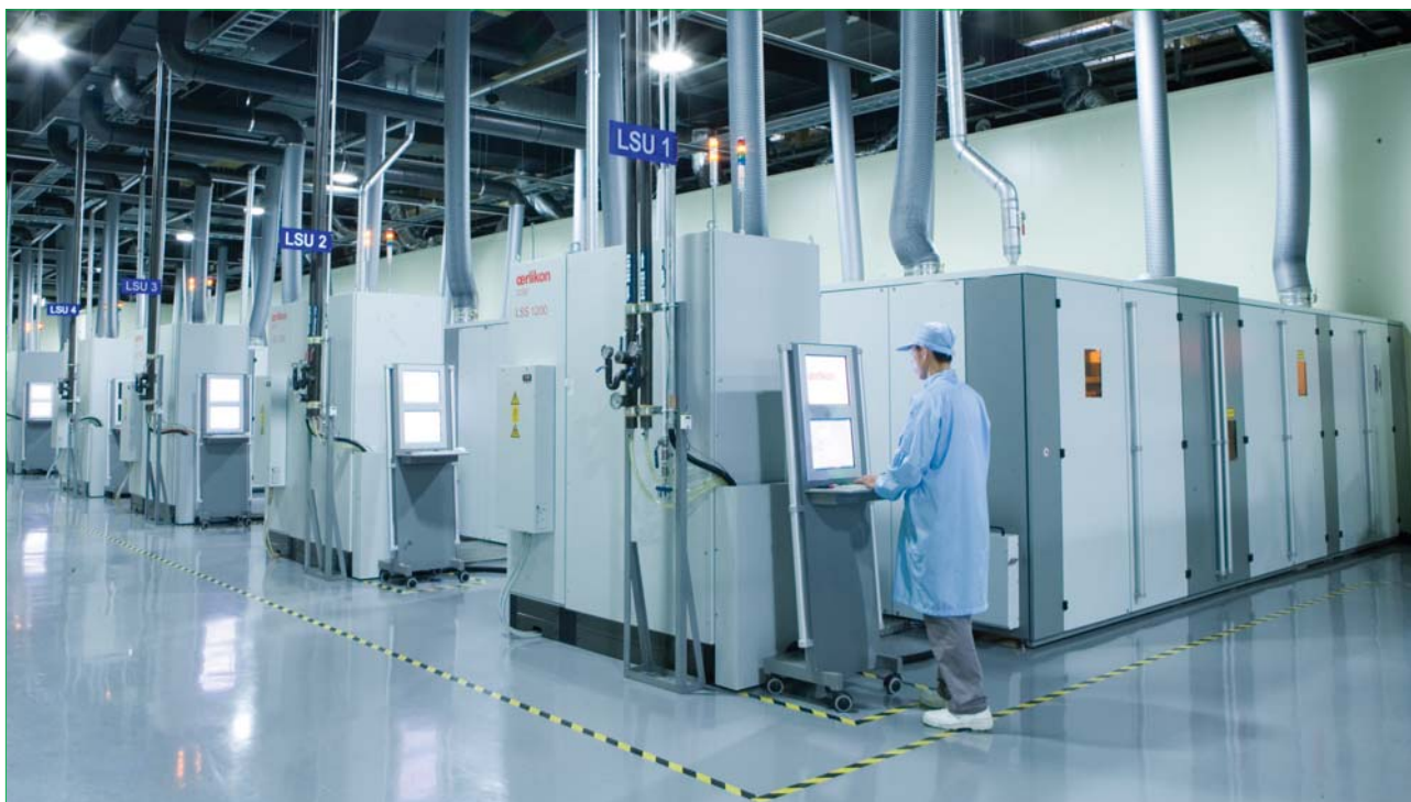
Figure 4. Laser-based tools within the solar industry are perhaps best represented by the thin-film patterning tools employed within turnkey Oerlikon thin-film production lines (image courtesy of Oerlikon Solar Ltd., Trübbach, Switzerland).
