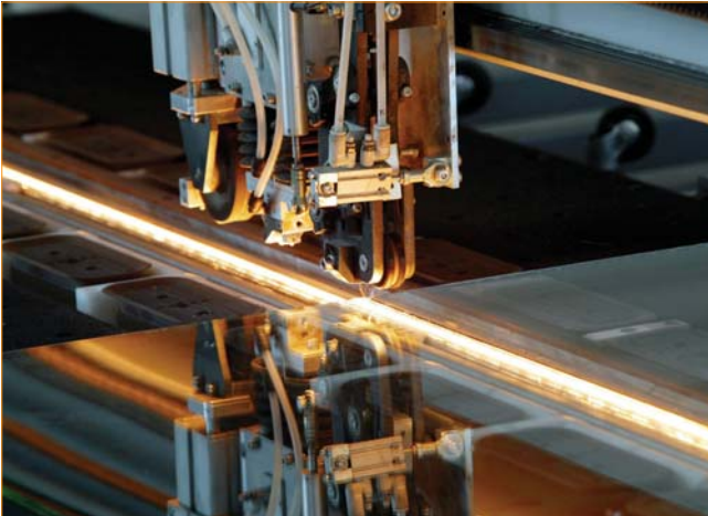
Figure 7. Solar glass also needs high-quality edges. Robotic devices operate at speed, guaranteeing precision.
