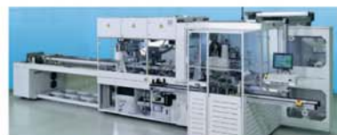
STRINGER TT – output 900 or 1200 cycles/h
