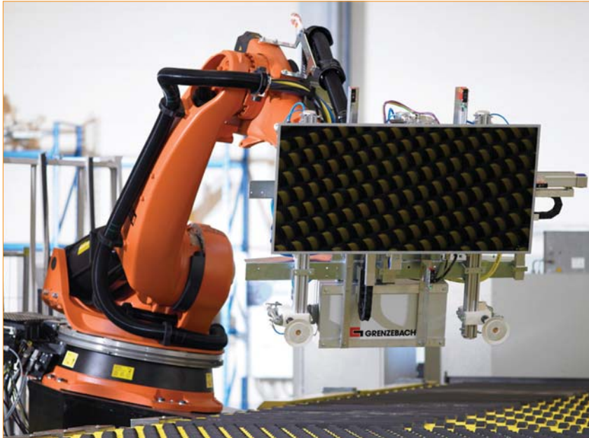
Figure 1. Robotic devices developed by Grenzbech, the German glass machinery manufacturer, take over contactless manufacturing of thin-film modules.
