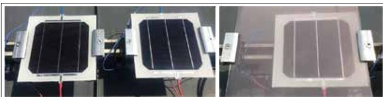
**Figure 8. PV mini module as a soiling-sensor with reference module for the investigation of the impact of dust accumulation on PV performance with monitoring of current, backside temperature, solar radiation; on the right the mini module with the artificial soiled anti-soiling coated glass [13]**
