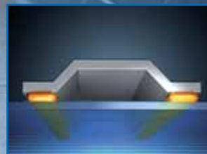
Bonding of back rails
