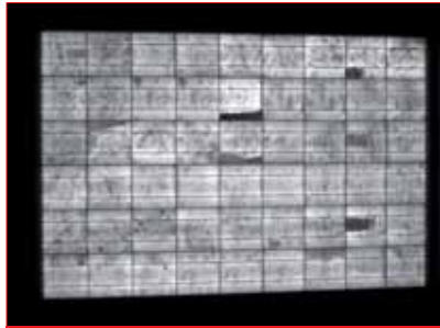
Figure 6. EL image – mc-Si module after the 2400Pa load test.
