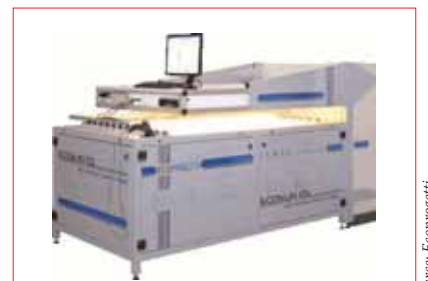
Ecoprogetti's ECOSUN10L sun simulator has received a triple class 'A' rating under EN60904-9 and IEC 60904-09 specifications.
