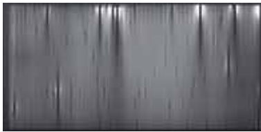
Figure 17. EL image – CdTe module (injected current = 0.1A).
