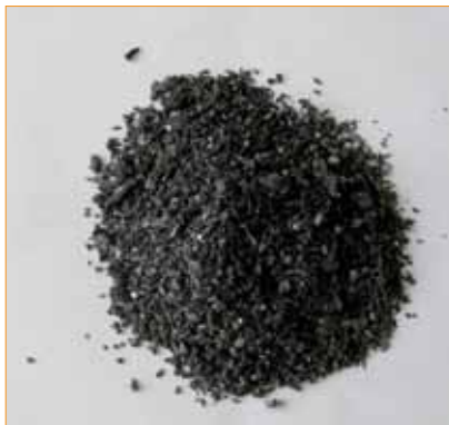
SiC is an agent for use in the high-precision ultra-thin slicing of silicon wafers.
