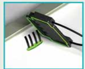
Junction Box Bonding and Ribbon Sealing
