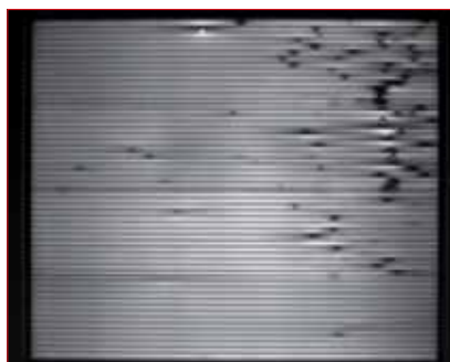
Figure 12. EL image – a-Si module after ageing.
