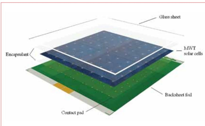
Figure 4. Back-contact module assembly using MWT solar cells.
