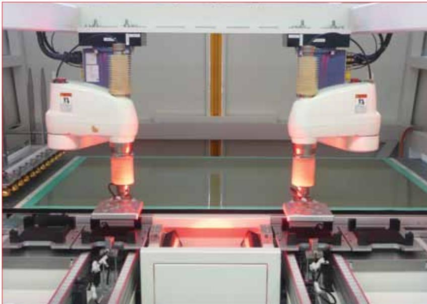
Figure 8. Close-up view of the pick-and-place robots.
