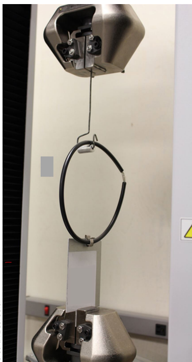
Figure 6. Wire clip mechanical load test
