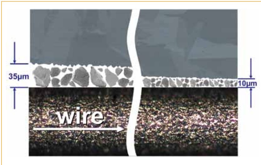
Figure 11. Collage of a wire beneath silicon and SiC particles in between the wire entry side (left) and the wire exit side (right) [12].
