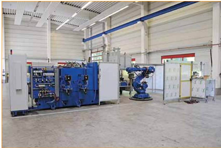
Figure 9. Fewer Si losses are possible through the optimal positioning of the block within the cropping saw.
