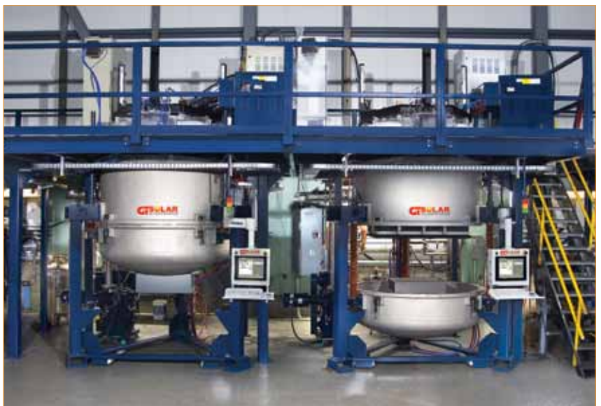
Figure 5. GT Solar's DSS450HP ingot growth furnace.
