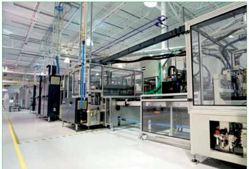
Figure 2. Automated back-end module assembly tools at the Longmont, Colorado manufacturing facility. These fully-automated systems have a throughput of approximately 65MW per annum.
