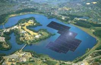
Kyocera Kyocera's 13.7MW floating PV array is expected to become the largest in Japan and the world
