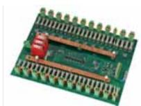
bloxx provides current measurements typically 10 times more accurately and is not susceptible to temperature variance. In addition, string voltage (up to 1,000V) and DC power on every string
