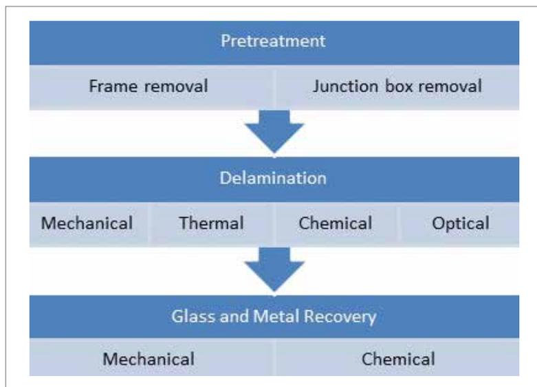
Figure 1. High value PV recycling process steps.
