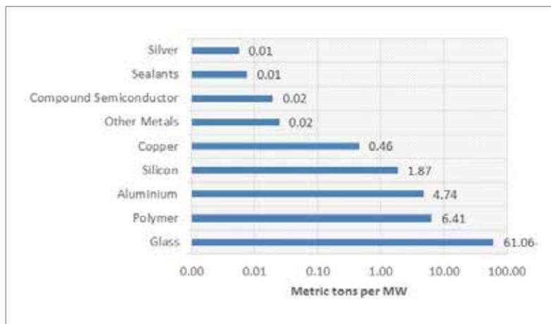
Figure 2. Average recoverable material fractions of PV Panels in 2030 based on [2].
