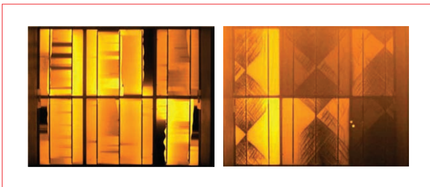
Figure 6. EL image of broken cells after in-laminate strength testing [5].
