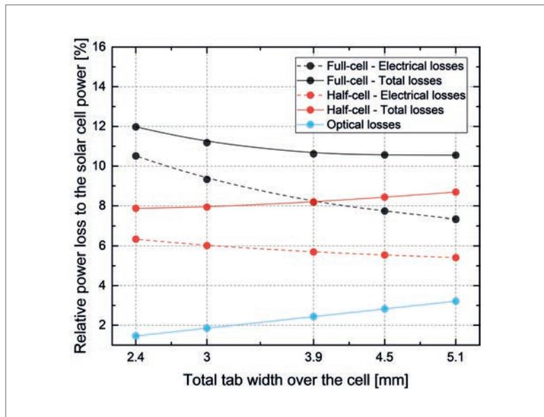
Figure 2. Electrical, optical and overall power loss of full-cell and half-cell mini-modules as a function of total tab width of all cell tabs, under standard test conditions (STC).
