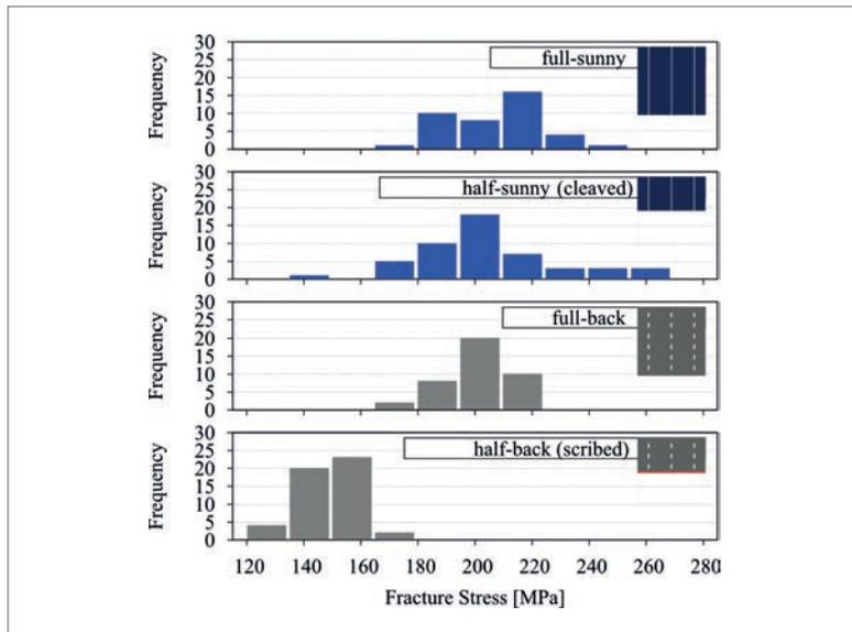
**Figure 4. Results for cell breakage frequency of full- and half-size solar cells, with fracture stress applied to the cleaved sunny side and laser-scribed back side of the cells. Significantly lower fracture stresses are observed when the cells are stressed on the laser-scribed edges.**
