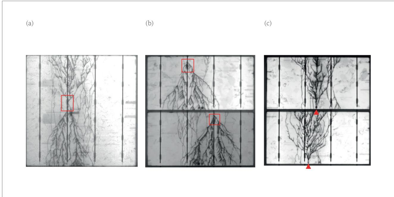
**Figure 6. EL images (contrast and brightness adjusted) of broken cells from the module laminate fracture tests, with fracture origin (red square) at the busbars for (a) full cells and (b) TLS, and at the cutting edge for (c) LSC [8].**
