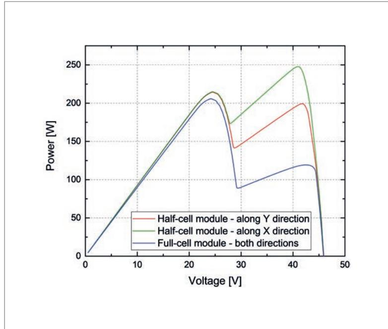
**Figure 8. Power–voltage curves for comparable half-cell and full-cell modules, when one solar cell or two half cells are affected by 70% shading in two different directions. The half-cell module shaded along the  $x$  direction still has all its strings in operation [14].**
