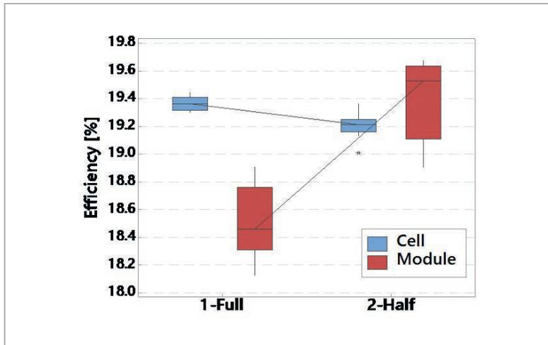
**Figure 3. Solar cell and module efficiency for full cells and half cells. While half cells have slightly lower efficiency than full cells, the effect is far more than offset at the module level under STC [11].**
