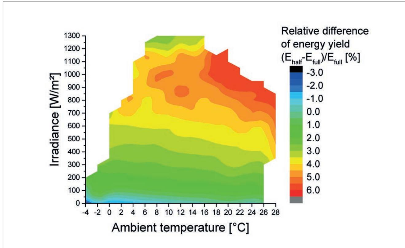
Figure 10. Relative yield gain of the half-cell module compared with the full-cell module  $(E_{\text{half}} - E_{\text{full}}) / E_{\text{full}}$ . The measured yield values for each module were summarized according to irradiation and temperature, and then averaged (intervals: 50W/m<sup>2</sup> irradiance, 2°C module temperature).
