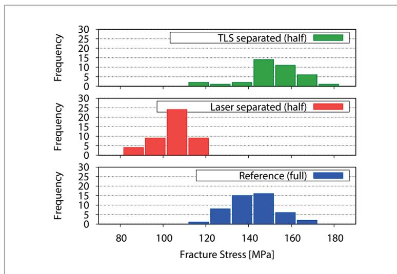
**Figure 5. Results for cell breakage frequency of full-size reference and half-size solar cells cut by thermal laser separation (TLS) and by laser scribing and cleavage (LSC). The TLS process often results in no detectable damage to the half-size cells.**
