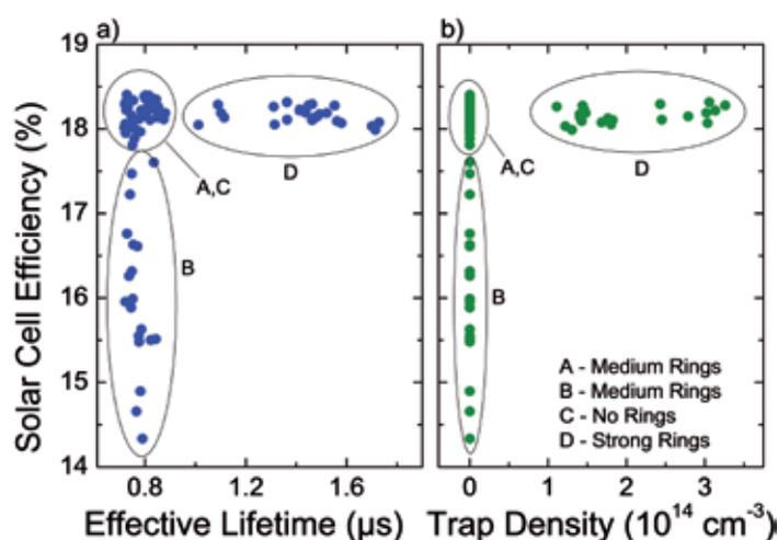
Figure 4. (a) Solar cell efficiency as a function of effective carrier lifetime, measured by means of QSSPC on the as-cut wafers; (b) cell efficiency as a function of trap density. Lifetime is limited by surface recombination and increased by charge carrier trapping, which may be corrected.
