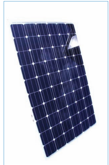
Figure 6. Photograph of a 60-cell module incorporating nickel/copper-plated solar cells.
