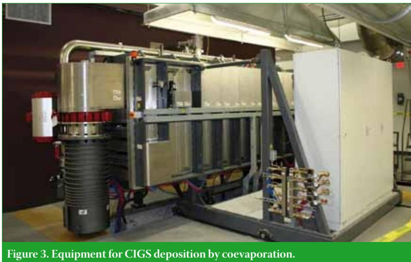
Figure 3. Equipment for CIGS deposition by coevaporation.
