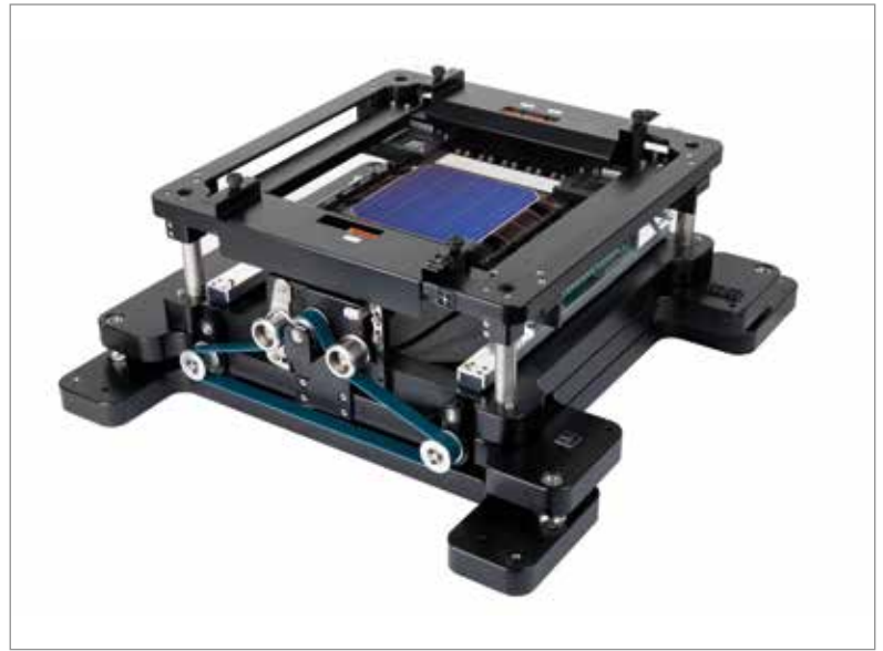
Figure 2. Grid TOUCH , PASAN's contacting unit for busbarless solar cell.
