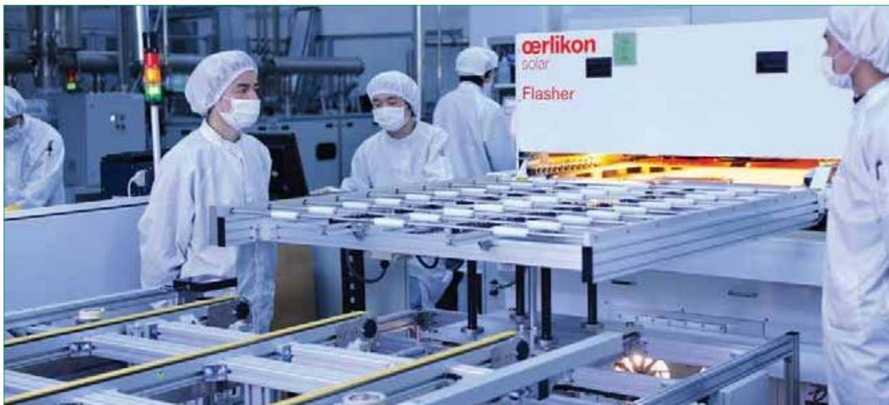
A dual-source solar simulator, with carefully tuned spectral balance, tests the tandem-junction panels.
