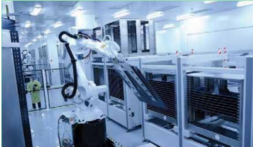
Astronergy's 30MW line is highly automated, employing a stocker-based approach.
