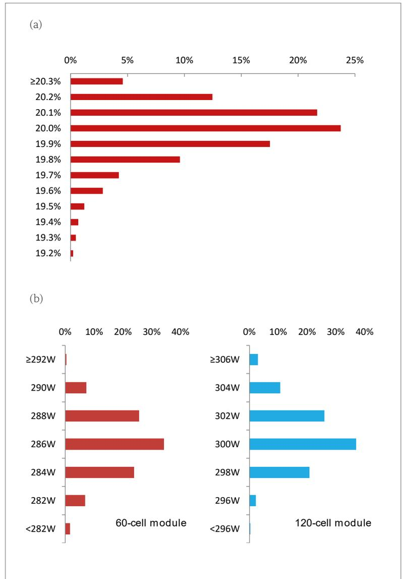
Figure 2. (a) Efficiency distribution of multi-PERC cells. (b) Wattage distribution of 60-cell and 120-cell multi-PERC modules.
