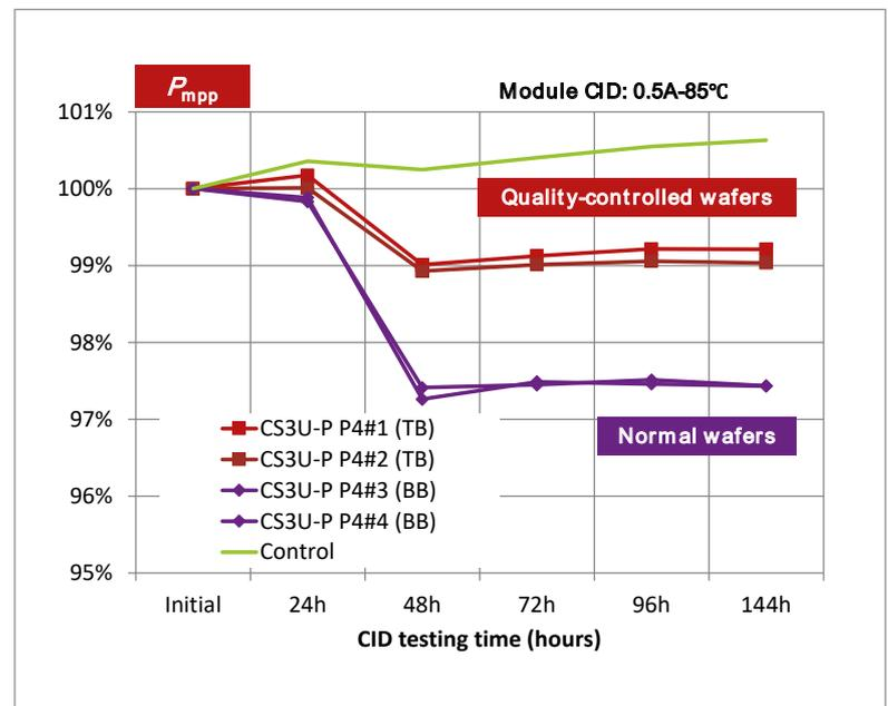
Figure 3. Effect of wafer quality on degradation performance of multi-PERC modules.
