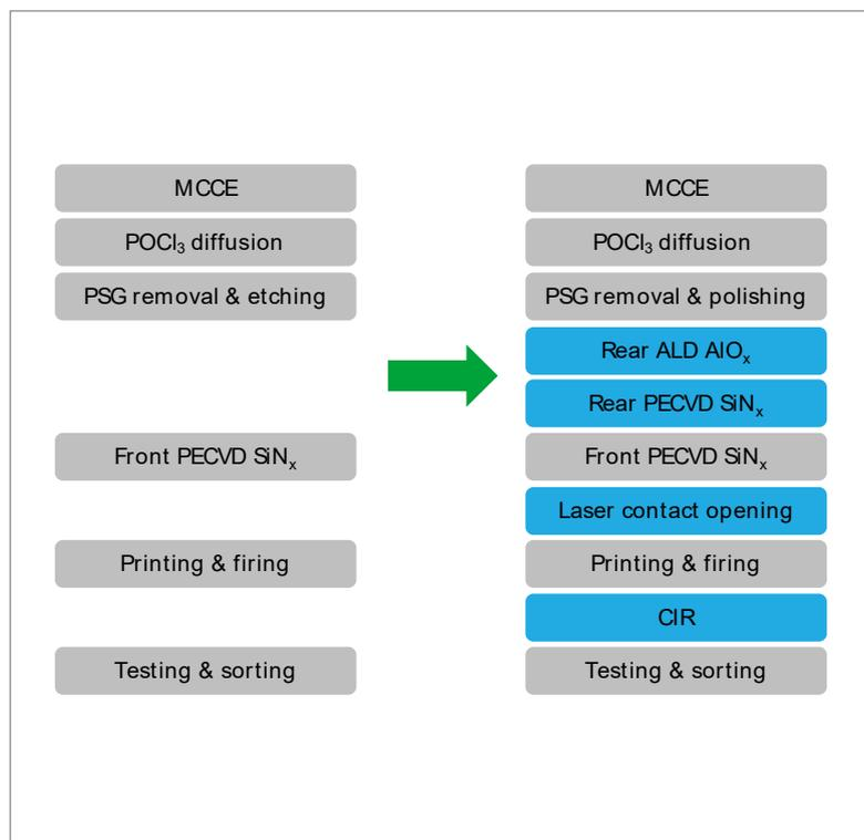
low-pressure  $\text{POCl}_3$  diffusion in the tube furnace. The next step is phosphosilicate glass (PSG) removal and rear-side polishing.
