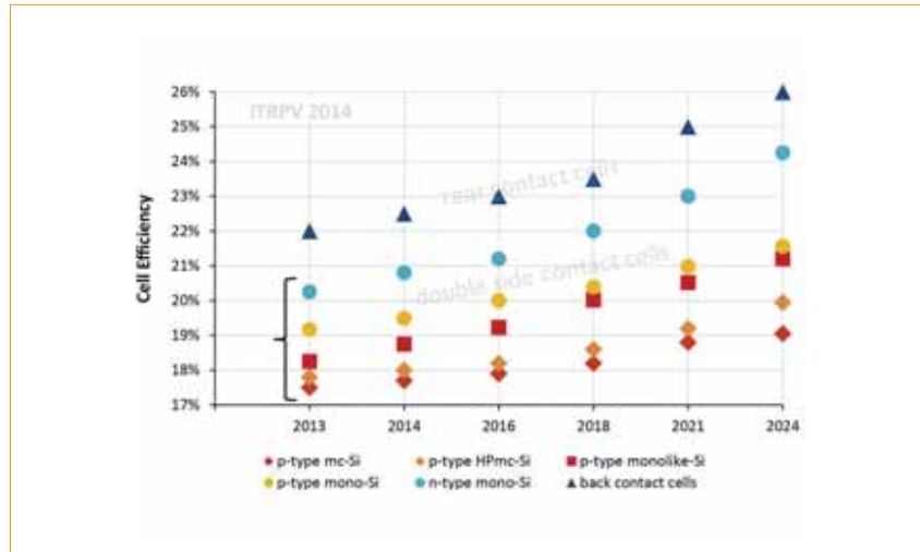
Figure 13. Stabilized cell efficiency trend curves for different c-Si cell concepts.
