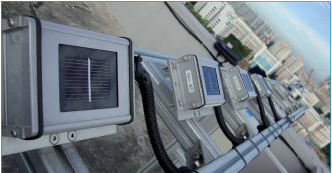
Figure 4. The irradiance measurement station located on the roof at the Solar Energy Research Institute of Singapore (SERIS).
