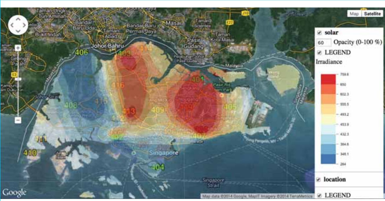
Figure 8. An interactive tool developed by SERIS, showing a live irradiance map taken at 12:00 noon on 1 February, 2014. Locations of the 25 irradiance measuring stations (numbered 401–425) in Singapore are shown. (Map: Google Maps, retrieved 1 February, 2014.)
